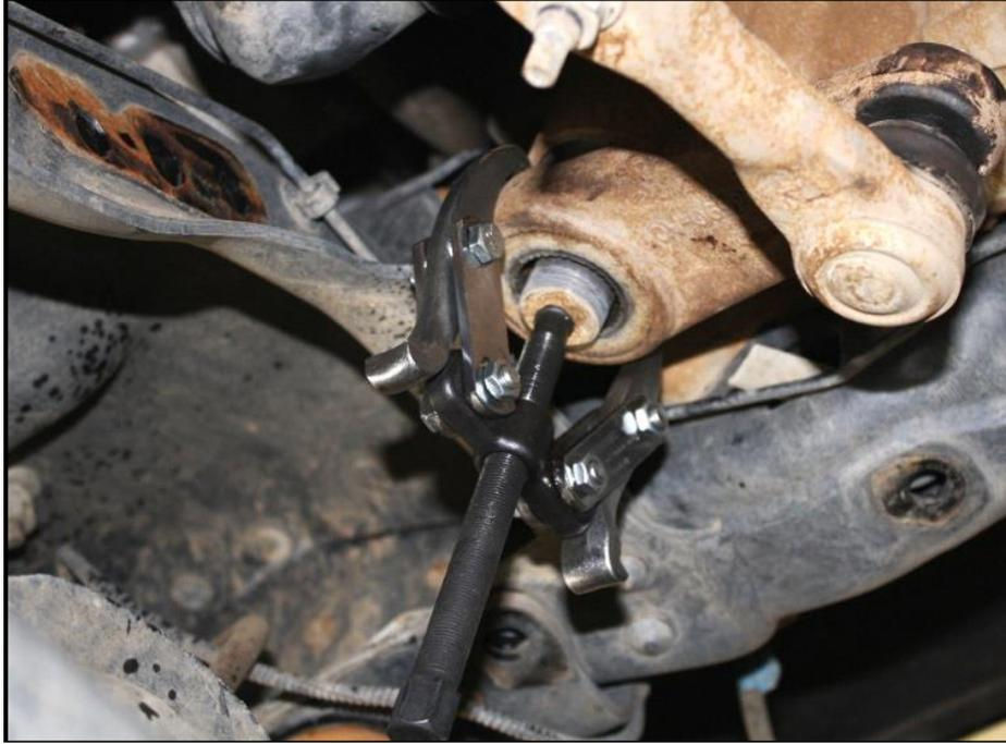
*Figure 5: Remove pitman arm from drag link.*
