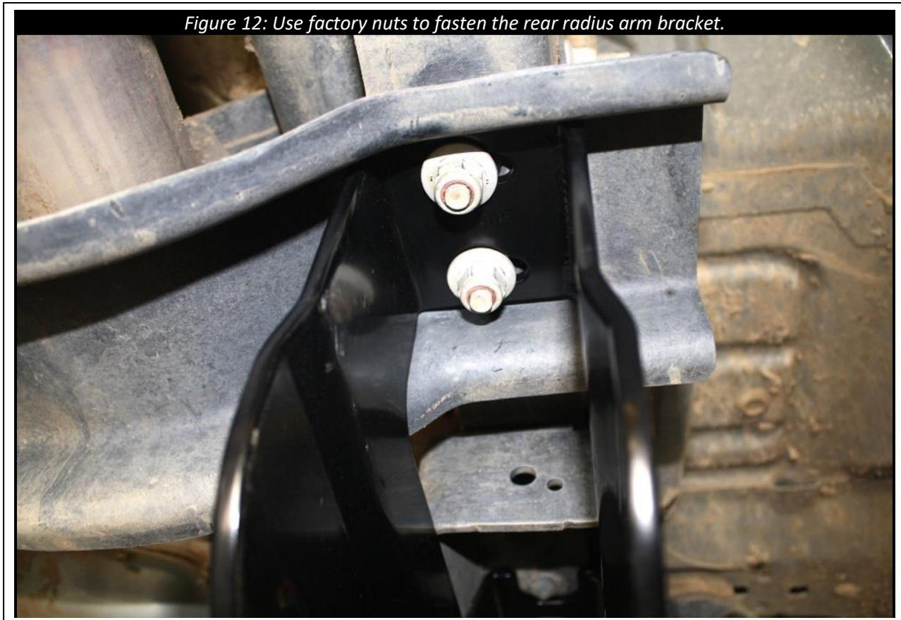
Install the radius arms into the drop brackets using the OEM hardware removed prior.
