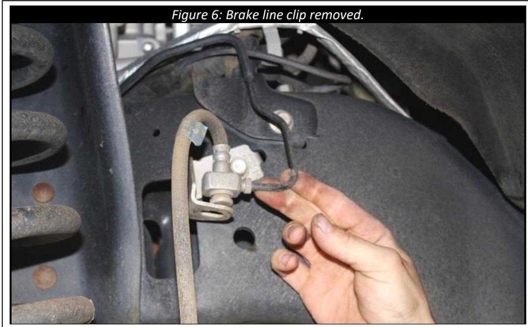
Remove the bolt restraining the mounting bracket to the frame, the bracket may be discarded but retain the hardware for reuse later.
