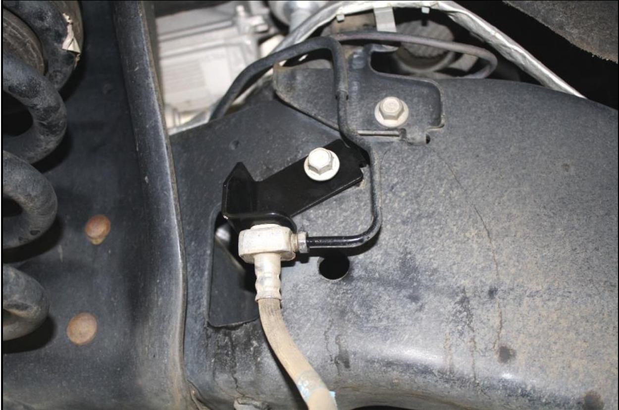
**16. Reroute the ABS wiring harness and attach to sensor:**
