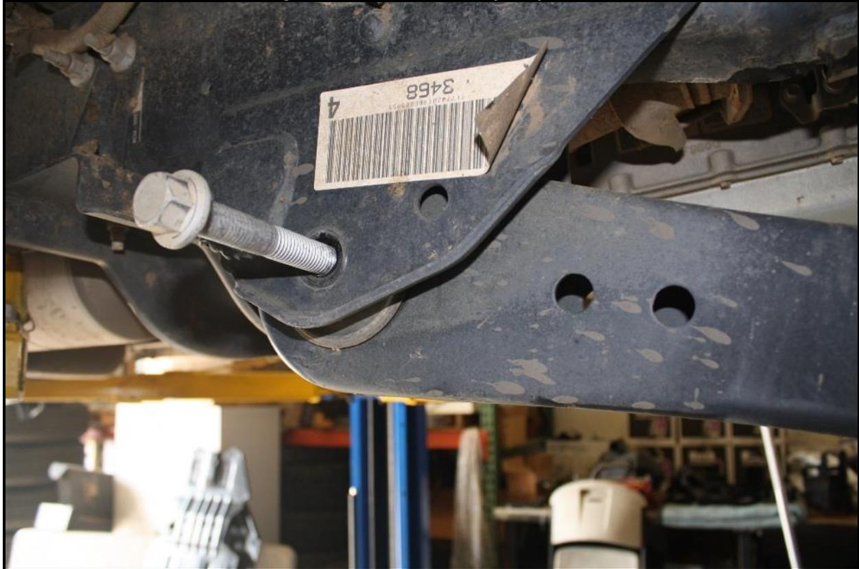
Remove any plastic clips that may be protruding into the mounting cavity that the radius arms were removed from. Support the transmission crossmember.
