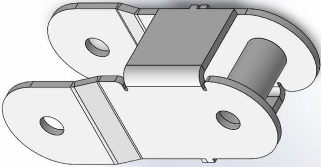
Figure 37: Driver Side Differential Drop Bracket.
