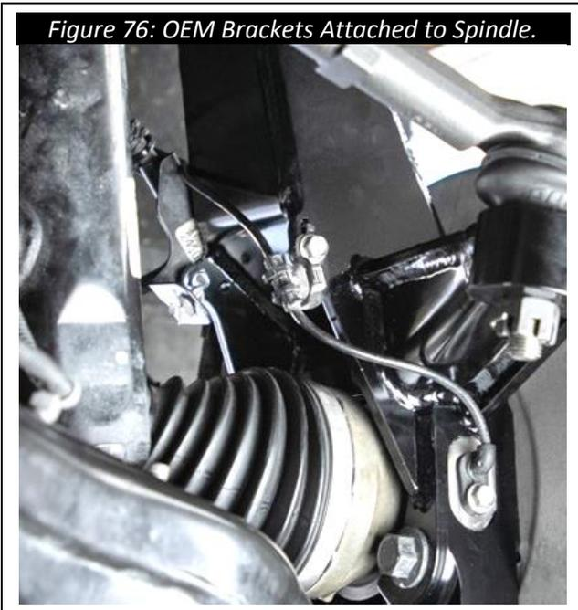
**Figure 76: OEM Brackets Attached to Spindle.**
