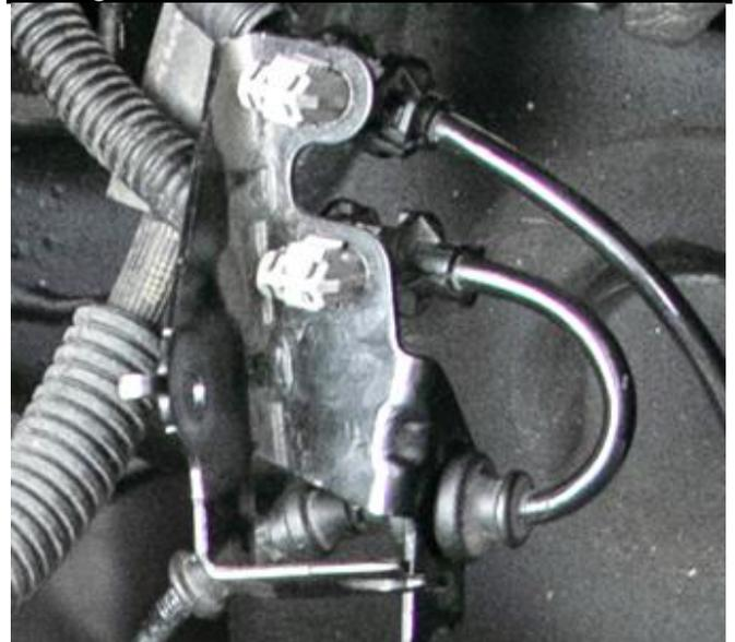
**53. Brake line and wiring routing:**
