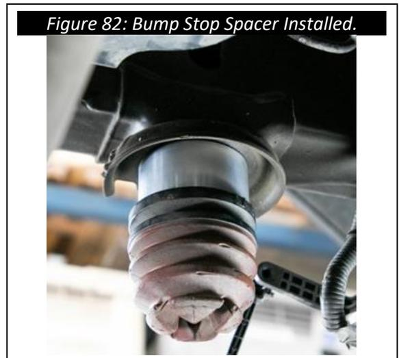
Figure 82: Bump Stop Spacer Installed.
