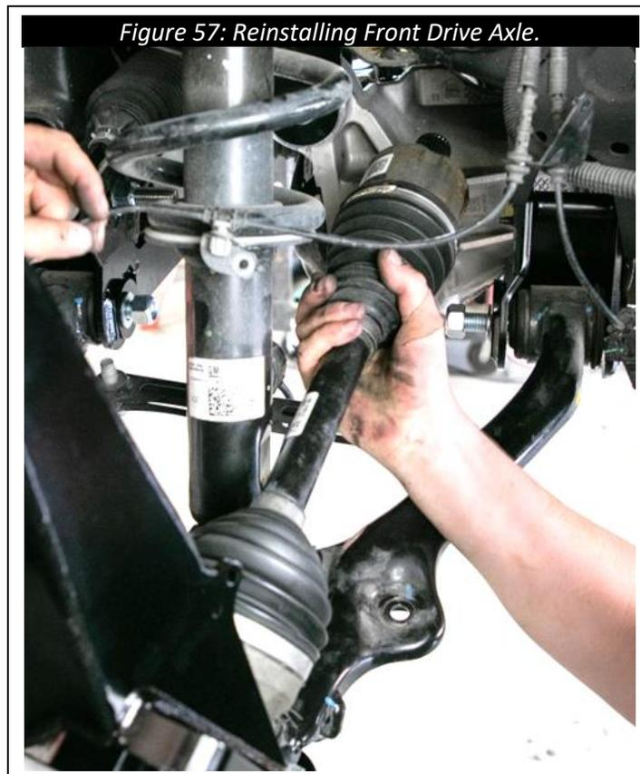
Figure 57: Reinstalling Front Drive Axle.
