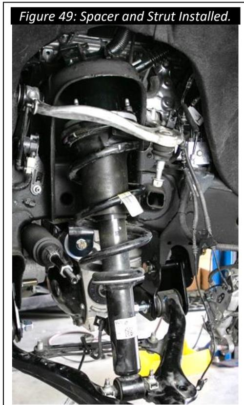
**34. Reinstall the lower control arm on both side of the vehicle:**
