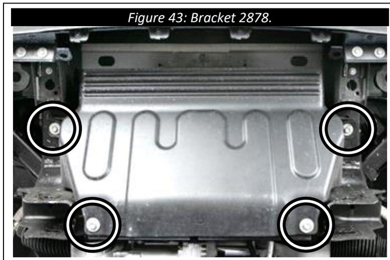
**31. Assemble the skid plate clip nut bars:**
