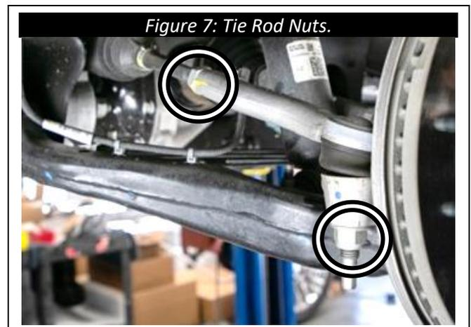
8. Separate the upper control arm from the spindle on both sides of the vehicle:
