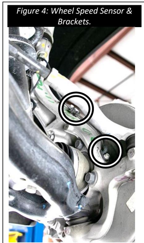
6. Remove the brake calipers with the brake pad wear sensors, if present, from both sides of the vehicle: Remove any brackets and hardware holding the brake line or sensor wiring to the spindle. Remove the bolts holding the brake caliper to the spindle. Hang the brake caliper from the frame, out of the way of work, set all hardware aside for reuse later.
