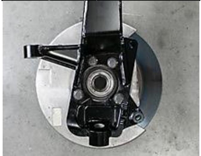
**37. Install the lift spindles on both side of the vehicle:**
