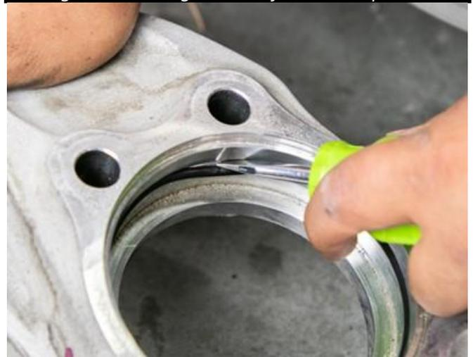
*Figure 55: Installing O-Ring into Lift Spindle.*
