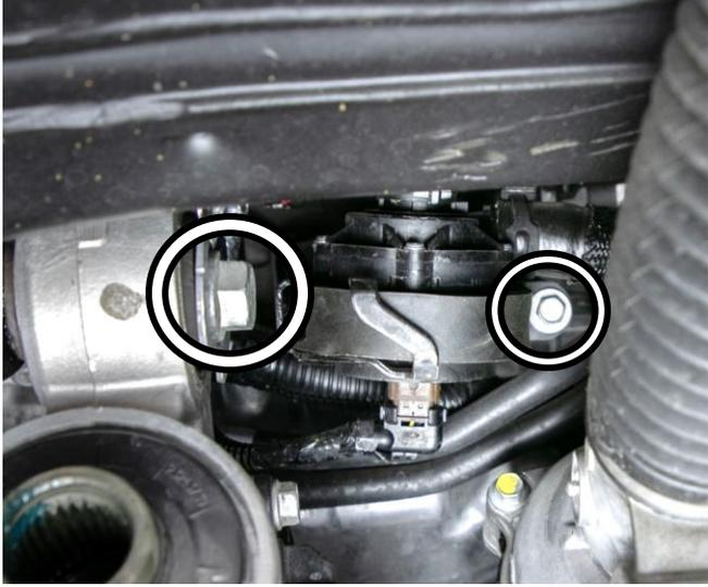
*Figure 18: Driver Side Differential Mount*
