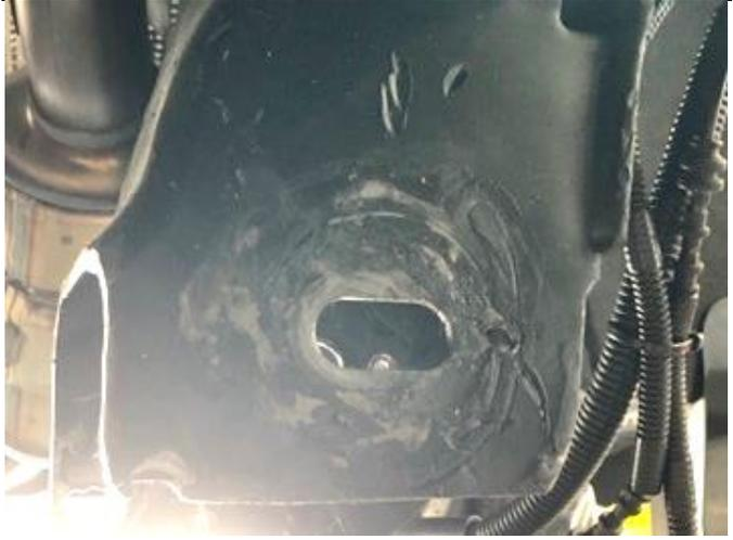
**Figure 25: After Trimming Passenger Side Crossmember.**
