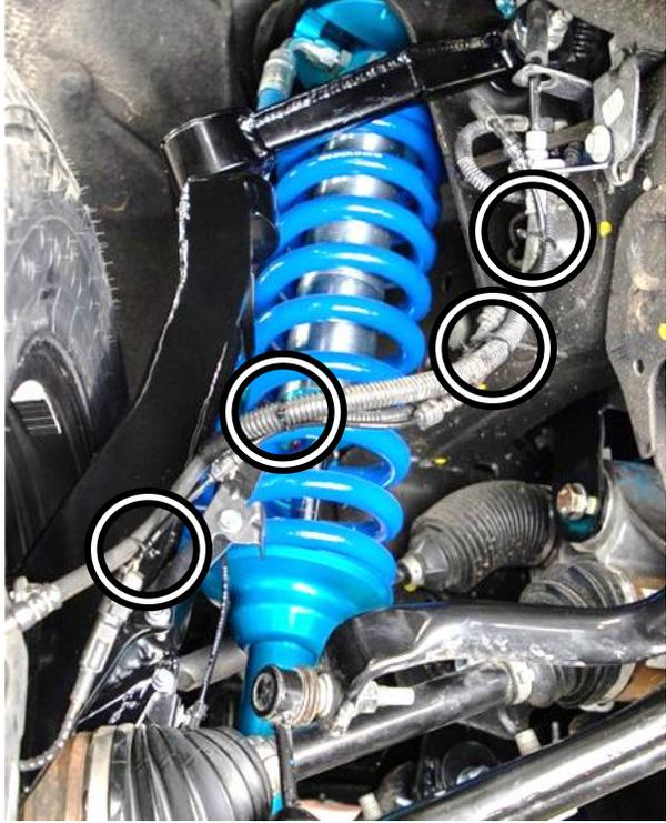
*Figure 74: ARC System Wire Routing.*
