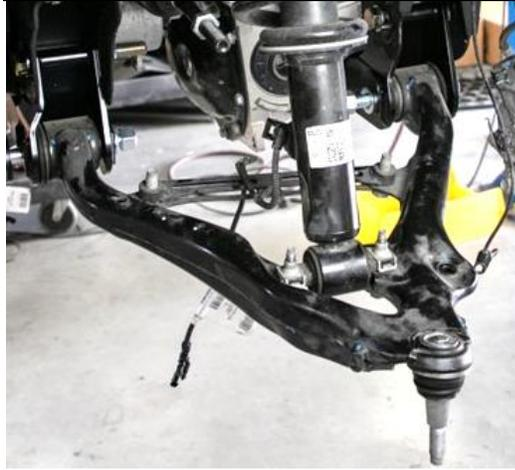
**35. Attach the strut to the lower control arm using the OEM hardware removed prior.**
