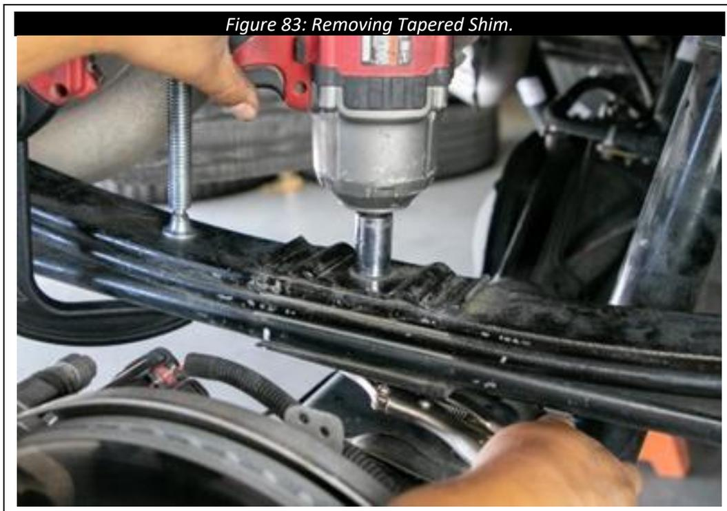
*Figure 83: Removing Tapered Shim.*
