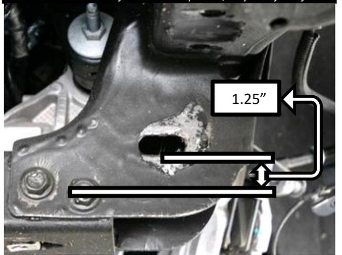
**Figure 24: After Trimming Driver Side Crossmember.**
