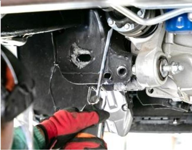
*Figure 21: After Cutting Crossmember Mount.*
