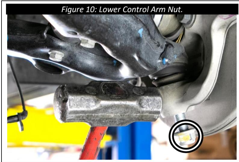
11. Remove the lower control arms from both sides of the vehicle: Remove the two bolts that hold the strut to the control arm, retain the hardware for reuse later. Remove the two bolts that mount the lower control arm to the frame, this hardware can be discarded. Pull on the lower control arms to free them from the frame, set them aside for reinstallation later.
