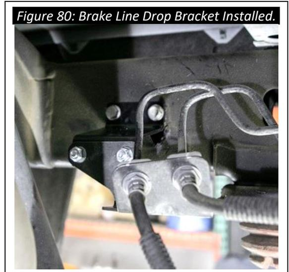
Figure 80: Brake Line Drop Bracket Installed.
