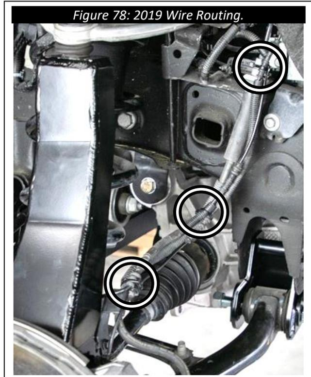
*Figure 78: ARC System Wire Routing.*
