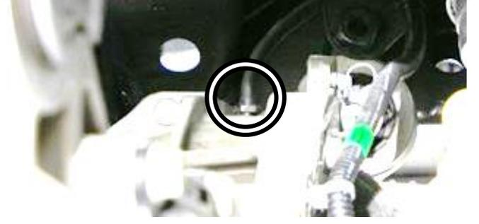
*Figure 20: Cut Driver Side Crossmember Mount.*
