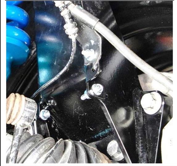
4. Remove Unused OEM Wire Routing Bracketry:
