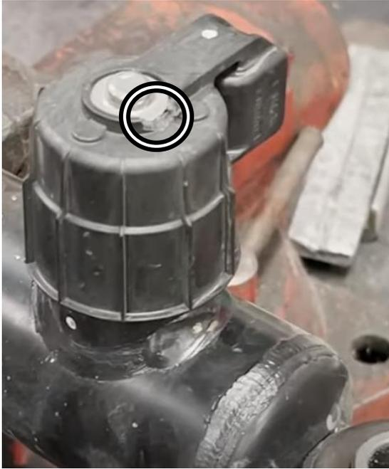
*Figure 2: Remove small metal cap.*
