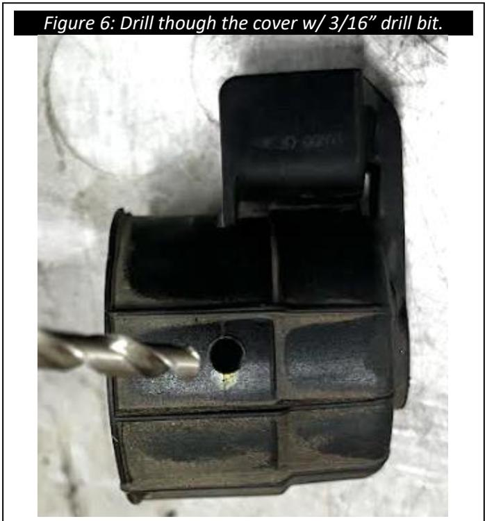
Figure 6: Drill though the cover w/ 3/16" drill bit.
