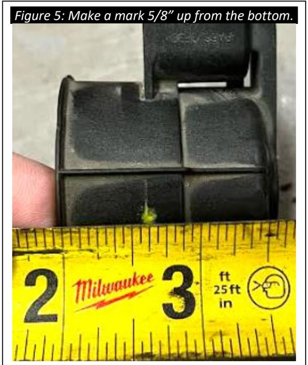
Figure 5: Make a mark 5/8" up from the bottom.
