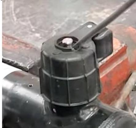
*Figure 3: Pull to remove plastic cap.*
