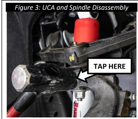
8. Remove the factory bolts and eccentric washers that connect the control arm to the frame and retain them for future use. Place them aside and note the order in which the components were removed, that way they may be re-installed in the same manner they came off. Remove the OEM Upper Control Arm (UCA) from the vehicle.
