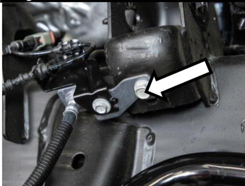
*Figure 2: Removing Brake Line Bracket and Wheel Speed Sensor*
