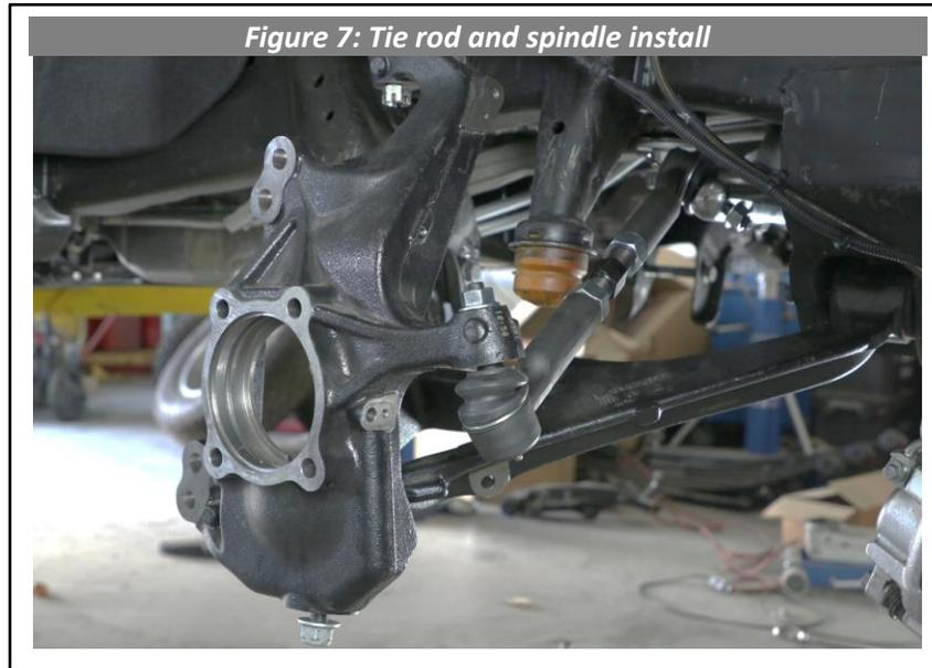
11. Adjust the tie rods with the center adjuster by using a **1" open end wrench**; **if you find that the tie rod assembly is too long, follow the instruction step below.**
