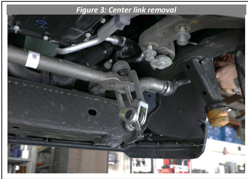
7. Locate the Cognito Billet Extreme Duty Center Link (PN 6529). One side of the center link has one additional hole for the steering stabilizer. This side will be installed towards the passenger side of the vehicle.
