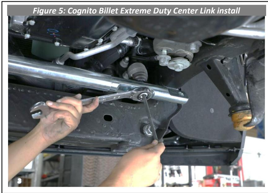
9. Remove the nut attached to the pre-assembled Cognito tie rod and insert the tie rod through the center link's tapered hole. Test fit the tie rod assembly. Fasten the nut back onto the tie rod and tighten hand tight.
