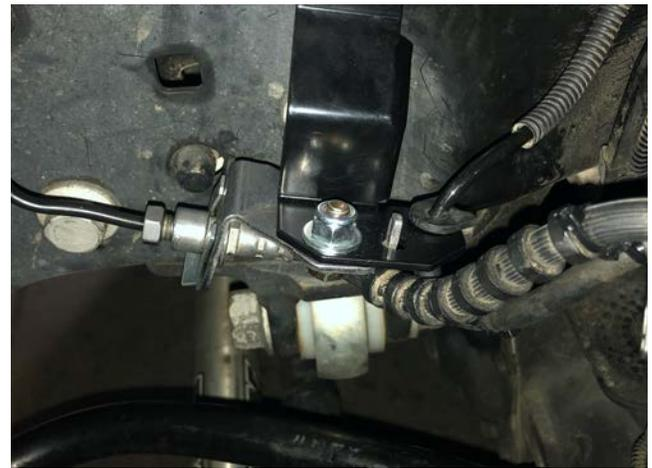
6. Once the brake lines are in place, turn the steering wheel all the way to passenger side of vehicle and check to make sure the brake lines are not interfering with springs, brackets, or tires. Repeat with the wheels turned all the way to the driver side of the vehicle.
