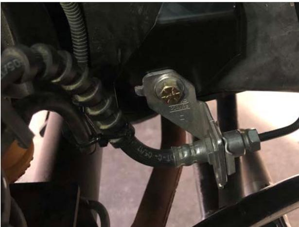
Figure 6: Driver Side ABS Line Routing
