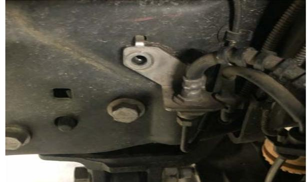
2. Remove the ABS line from both driver and passenger side OE brake line brackets by pulling the rubber boot out of the containment slot (Figure 2 A/B).
