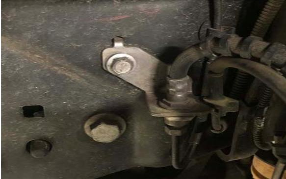
*Figure 1B: OE Brake Line Bracket, Bolt Removed*
