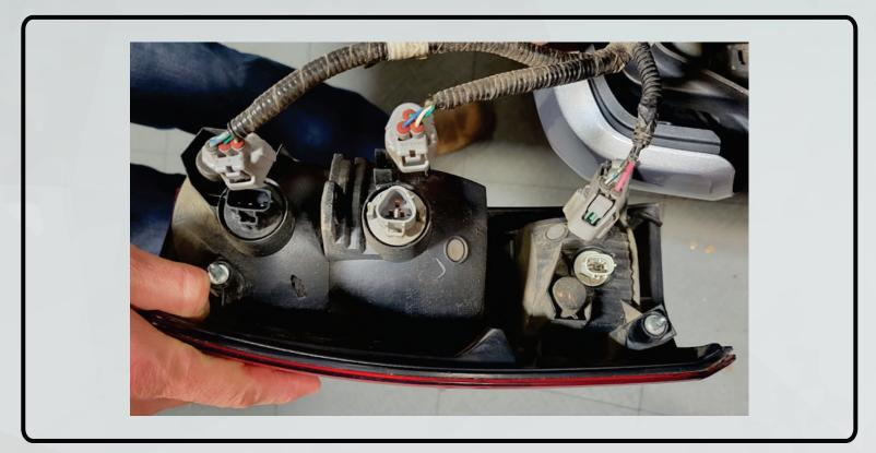
3. Determine which style turn signals you would like from your tail lights. Connect red + green for sequential turn signals or red + yellow for standard on/off turn signals.
