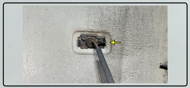
5. Remove and transfer the stock foam gasket to the new Morimoto marker lights.
