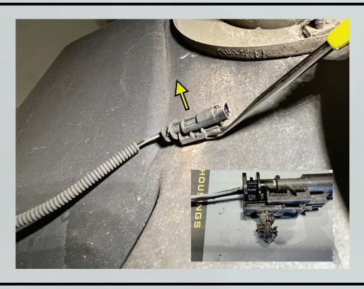
3. Pry the release tab up to pull the factory press clip off of the connector. This clip will be reused.
