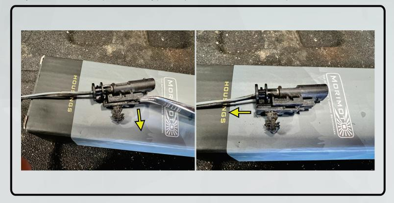
4. Press in the side tab to release the stock side markers. The side marker then removes from the front (painted side).
