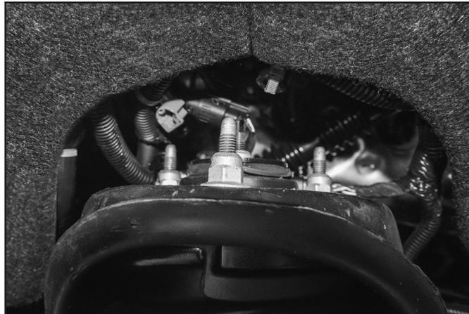
11. Remove the ABS wire / brake sensor wire from the upper control arm. Remove the upper control arm from the vehicle by removing the two bolts attaching the upper control arm to the strut bucket / frame (Fig. 8). If replacing the upper arm on a Denali truck, remove the sensor arm from the ball stud on the upper control arm.
