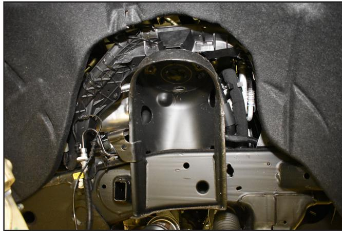
12. The new replacement control arm assemblies have a larger profile than the OEM assemblies. They are also designed with a wider range of available travel. Due to these unique differences, the tab on the side of the strut bucket must be removed to avoid interfering with the proper function of the new control arm assembly. Cut the tab from the side of the strut bucket as shown in Figure 9.
