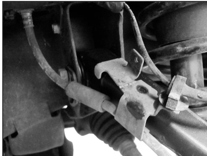
6. Disconnect the brake line bracket from the upper control arm. Hardware will not be reused.
