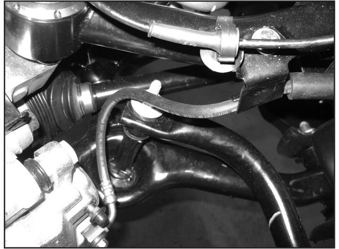
17. Reattach ABS wire to factory mounting clips and brackets. It may be necessary to slide the ABS wire in the rubber grommets to get adequate clearance / routing of the wire. Use silicone spray to allow the grommet to slide on the ABS wire.
