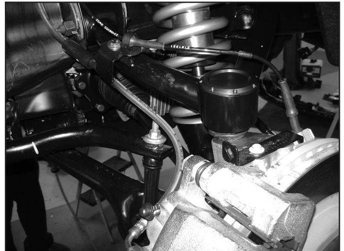
16. Attach modified factory brake line bracket to the upper control arm with ¼" hardware. Tighten to 12 ft-lbs. Cycle the steering to ensure that the brake line clears the sway bar components. Rotate bracket if necessary. (Fig 8a, 8b)
