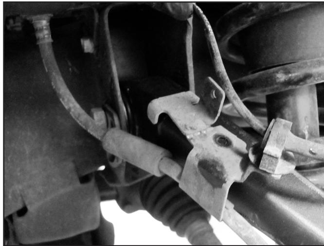
6. Disconnect the brake line bracket from the upper control arm. Hardware will not be reused.
