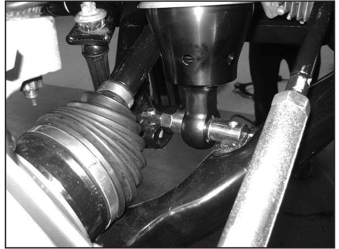
13. Attach the upper control arm to the steering knuckle with included castellated nut. Tighten to 45 ft-lbs, install cotter pin.
