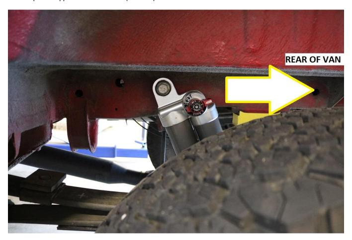
5) With the top of the shock bolted into the upper mount, ensure the shock shaft is extended out all the way. Adjust the SP2 mode adjust by rotating the shaft 360 degrees in the direction as specified below for the corresponding van weights:
