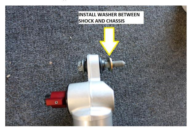
4) Be sure to orient the shock body so the reservoir is positioned towards the rear and the adjuster faces out. Torque the upper bolt to 100 ft-lbs (108 N.m).
