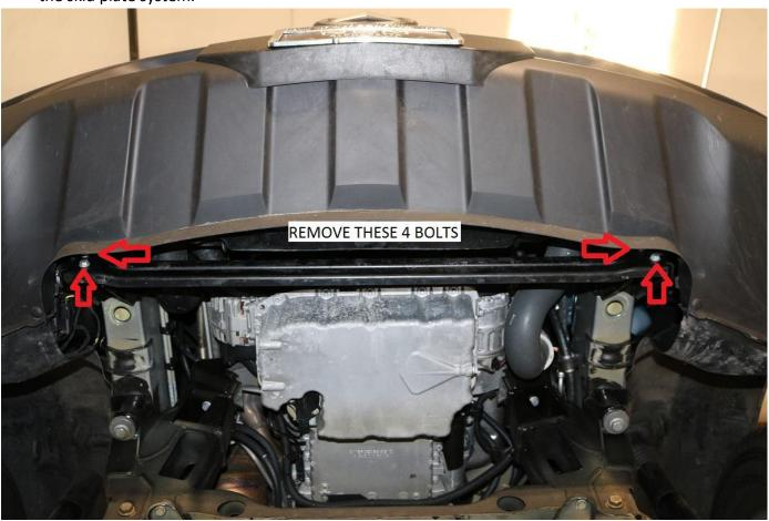
3) Remove the front sheet metal guard from the vehicle.
