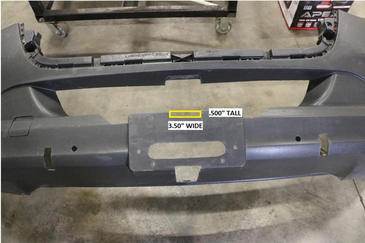
40) Drill the fairlead holes out to at least  $\frac{1}{2}$ " (13mm) in diameter. Use a Dremel style tool or pneumatic die grinder to cut out center slot. Example of finished cut is pictured above.
