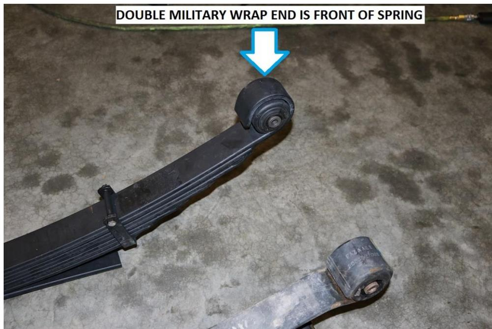
14) Install the leaf springs into the vehicle. We have found it easiest to install the springs upside down and then rotating them up into position once under the vehicle.
