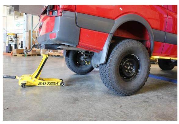
2) With the factory shocks removed on both sides of the vehicle, locate the bolt securing the Emergency brake cable to the PASSENGER side rear lower shock mount. Remove this bolt / nut using a 16mm socket / wrench. Retain the OEM nut as it will be re-used.
