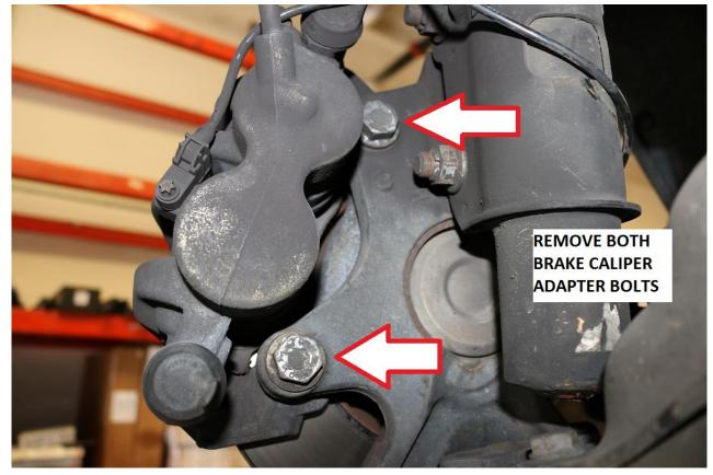
22) Remove the brake caliper from the rotor and secure up out of the way. Do not allow the caliper to hang by the brake hose.
