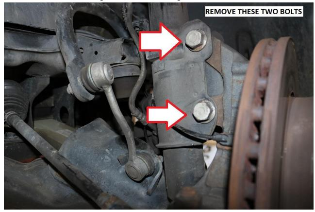
24) With the strut disconnected from the steering knuckle, allow the lower control arm to hang free again. Be careful to slowly lower the knuckle out of the strut. Be sure the wheel speed sensor wire is not strained.
