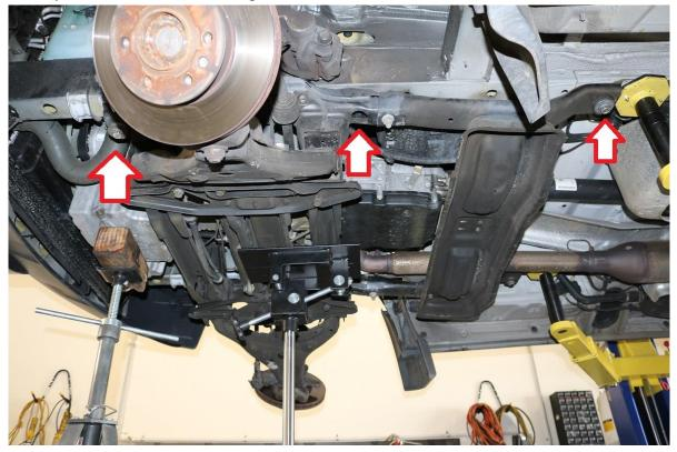
40) Prepare the spacers and new sub frame attachment bolts. The image below shows where each bolt / spacer is designed to be installed. It is critical to use the correct bolts / spacers in their corresponding locations.
