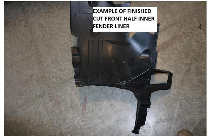
90) Cut the rear half of the inner fender liners as shown in the images below.
