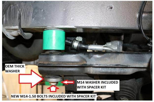
44) Snug all 6 bolts but do not torque at this time. Final torqueing will occur once the motor mount spacers are installed and the engine / transmission support jacks & jack stands can be removed.
