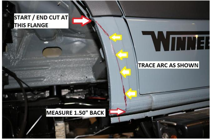
81) Continue the cut on the inner pinch seam. The cut should leave approximately 3/8" (9-10MM) of pinch seam left at the bottom. See image below.
