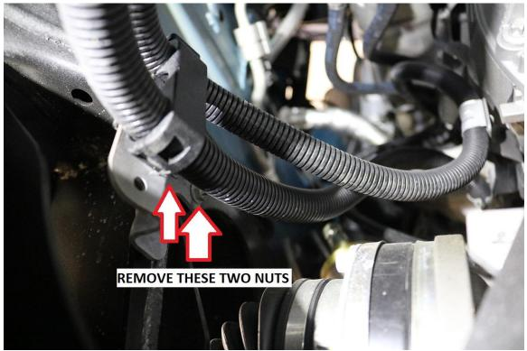
36) With the bracket separated from the chassis, use a small flat blade screw driver to pry up under the plastic retention clip so the bracket can be freed from the cables.
