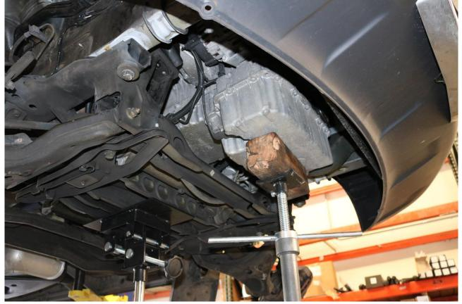
30) Remove the motor mount bolt on both the driver and passenger side with a 16mm socket / wrench.
