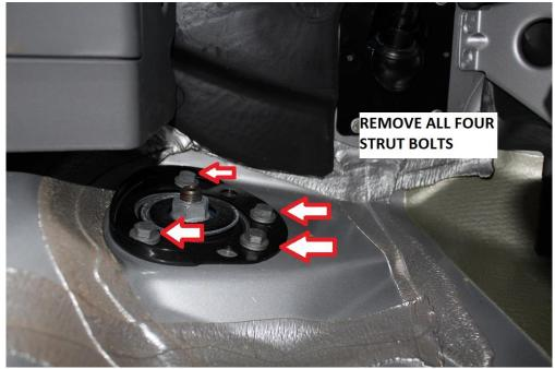
26) The passenger side upper strut bolts can be accessed by pulling up the tool kit cover panel in the passenger footwell. Use a large flat blade screwdriver to rotate the lock knobs on the kick panel so they are horizontal.
