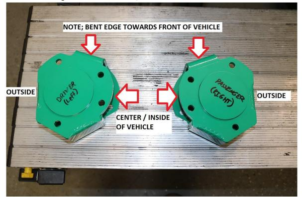
59) Install the spacers onto the top of the struts using the OEM strut bolts originally removed. Snug all bolts tight, and add an additional ¼-1/2 turn. The torque spec on these bolts is only 21 ft-lbs (28 N.m).
