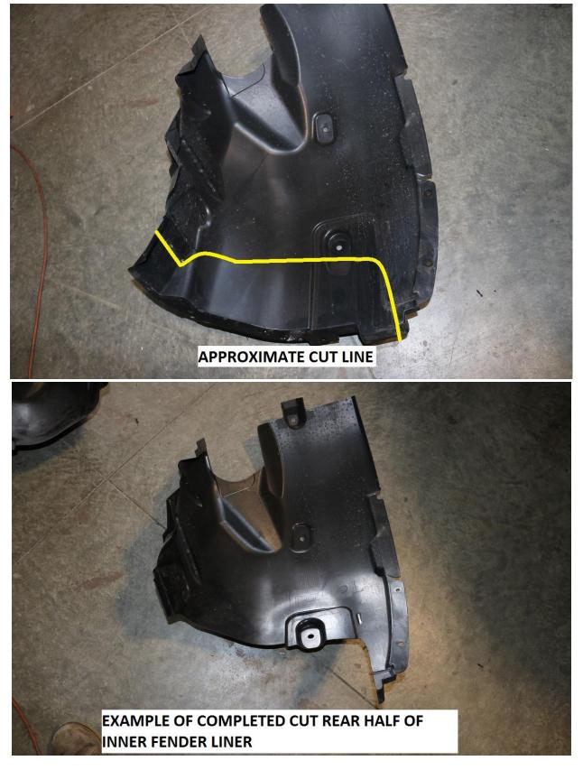
91) Install trimmed fender liners and mudflap as shown below.
