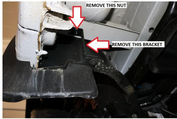
79) Remove and retain the clip on nuts which secured the mudflap to the rear of the front fender.
