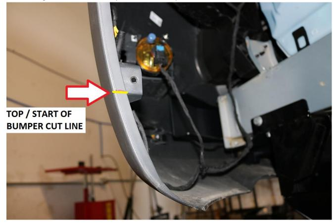
86) From the line marked in the previous step, continue cut line down so it is tangent with the bottom outer push pin hole in the front bumper cover. See image below for reference.
