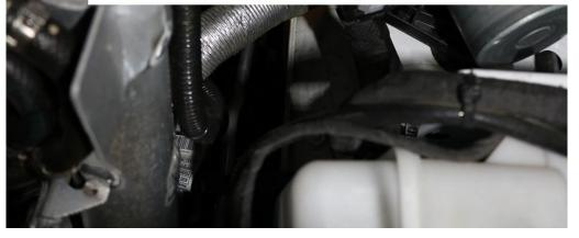
7) Locate the low pressure power steering hose going from the steering rack to the power steering cooler. See image below for reference.
