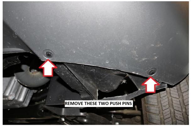
13) Use an automotive trim removal tool to pry up under the head of the push pin prior to prying under the body of the fastener to fully remove it.
