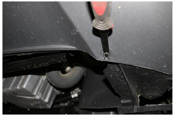
14) Next, on the inside of the fender well, remove the three push pin fasteners near the outer lip of the bumper.
