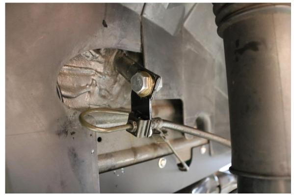
74) Orient the tab as shown above. Tighten the M12 bolt to 50 ft-lbs (67 N.m). Reconnect the hard line to the brake hose and snug the brake line fitting tight.
