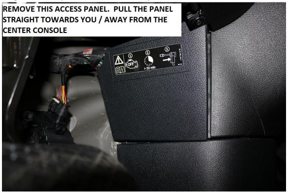
3) Remove the access panel and locate the ground cable. Press down on the red tab to release the lock tab and pull the connector back away from the firewall. Position the ground cable so it will not touch the grounding post for the duration of this installation.
