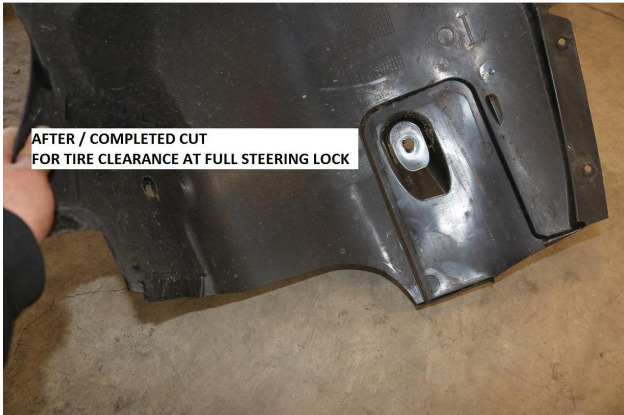
61) Re-install the fender well liners in the reverse order of removal.
