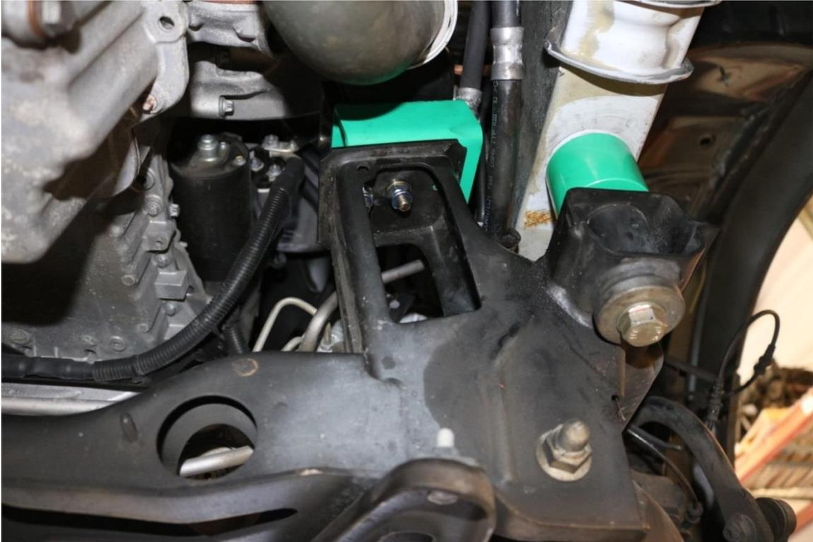
48) At this time, torque the transmission mount bolts to 22 ft-lbs (30 N.m)
