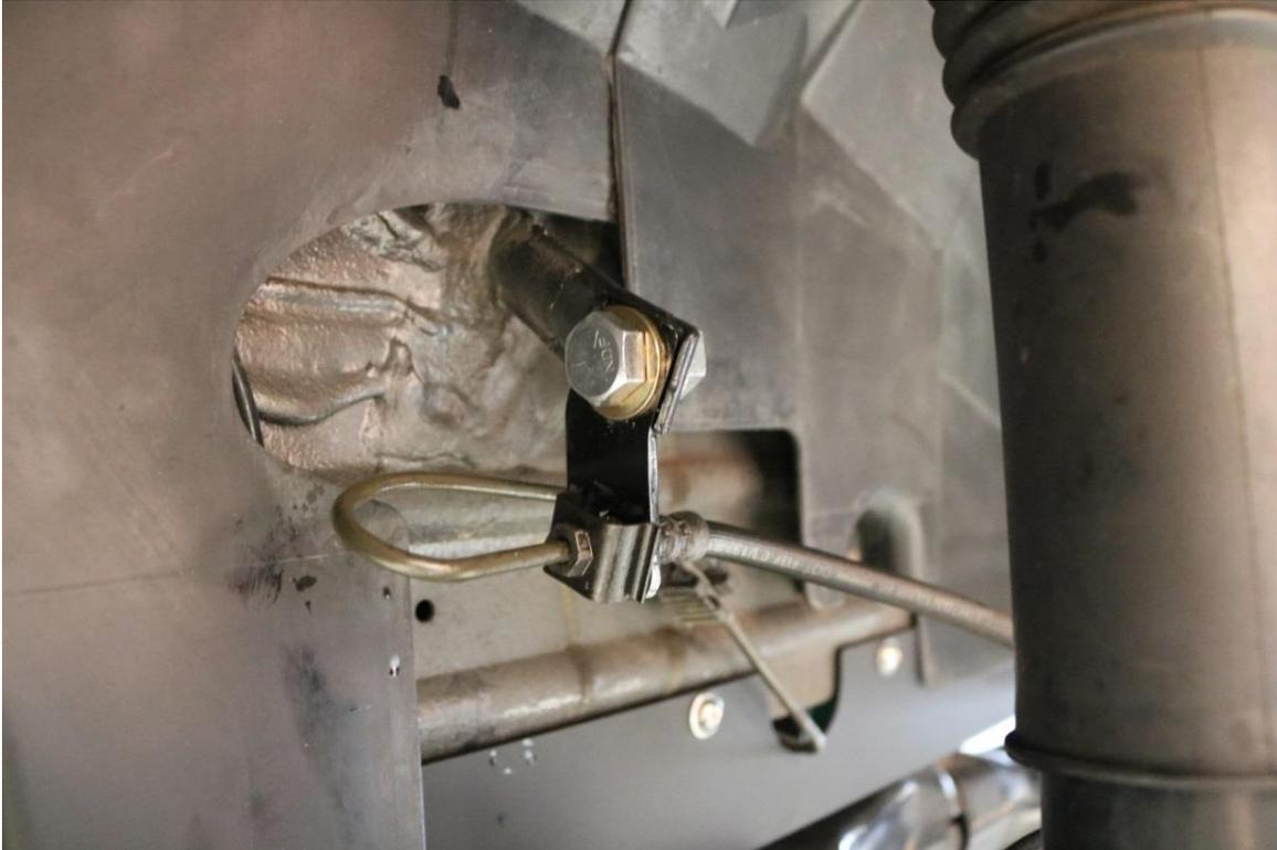
67) Orient the tab as shown above. Tighten the M12 bolt to 50 ft-lbs (67 N.m). Reconnect the hard line to the brake hose and snug the brake line fitting tight.
