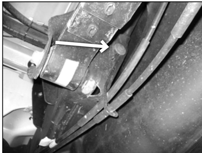
6. Remove the ABS wire clips from the metal tabs just inside of the leaf springs. Remove the plastic clips from the ABS wire. (Fig 2)
