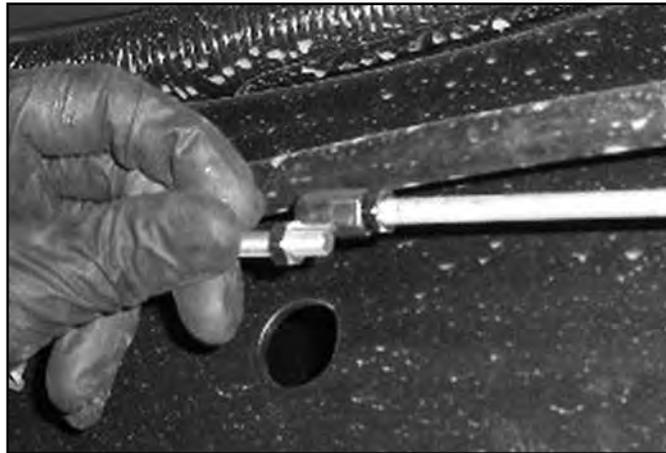
18. Attach the M6 threaded extension (SBTE) with jam nut and tighten securely.
