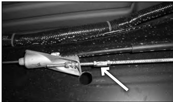
20. Reinstall the E-brake cable bracket near the jounce bumper with factory hardware.
