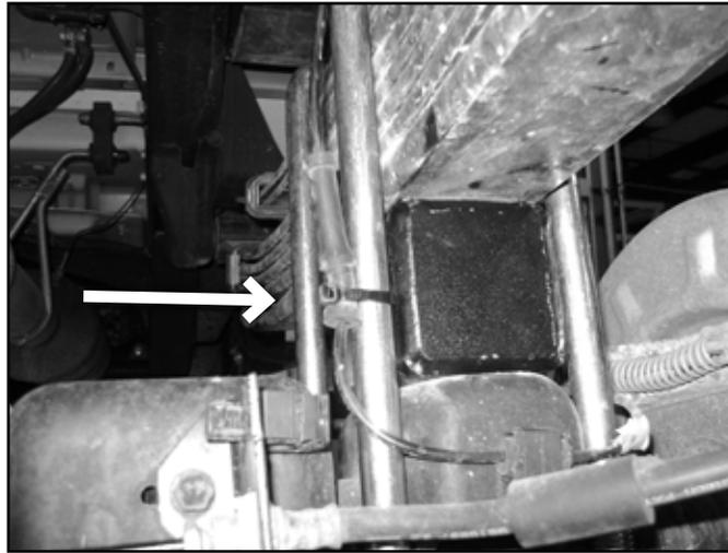
14. Check all cables for adequate slack at full droop, make adjustments if necessary.
