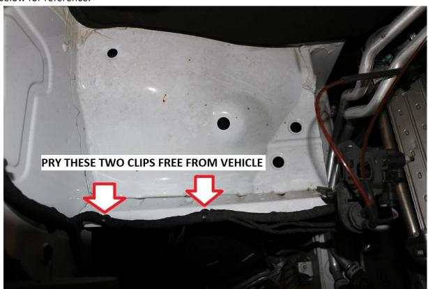
4) Remove the front passenger side inner fender liner by first removing the two push pins located near the front bottom side of the bumper. See image below.
