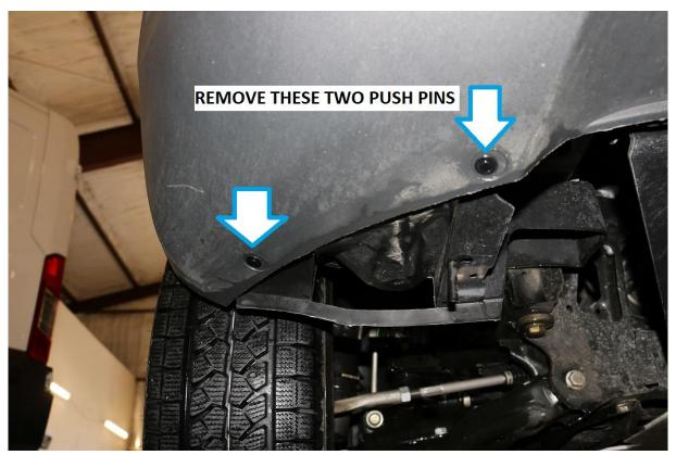
5) Use an automotive trim removal tool to pry up under the head of the push pin prior to prying under the body of the fastener to fully remove it.
