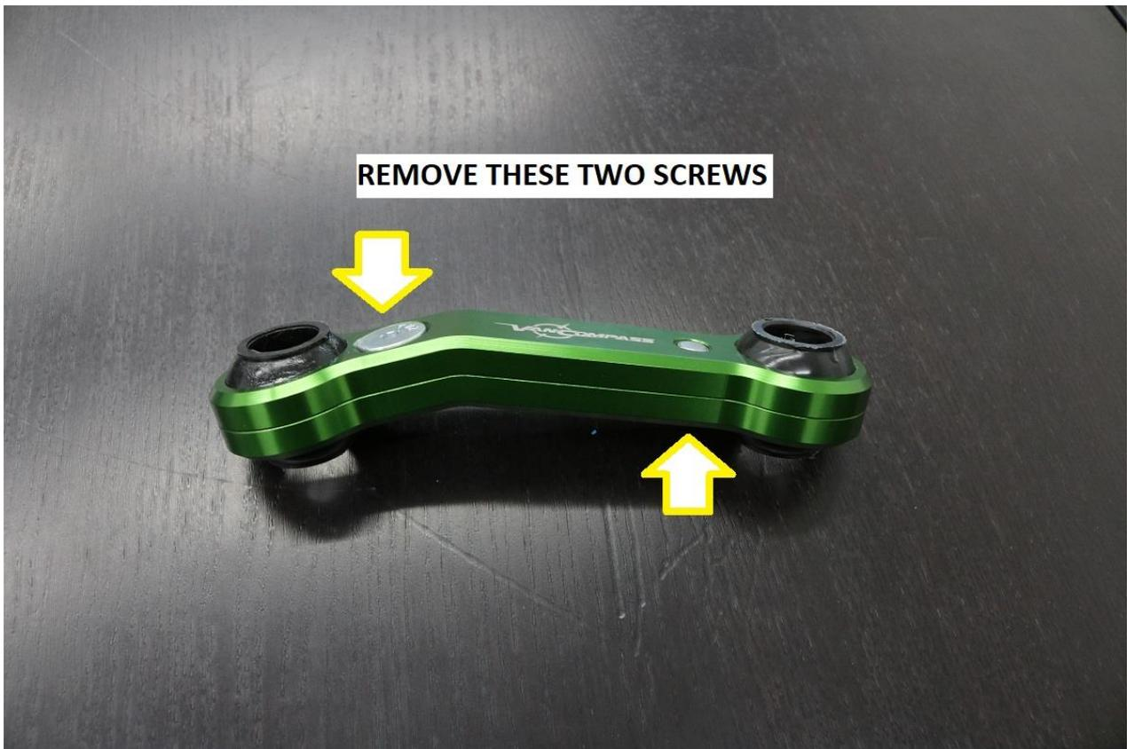
3. Thoroughly clean all the components. Re-grease the bushings as described below with a quality chassis grease such as Lucas Red N Tacky #2 grease.
