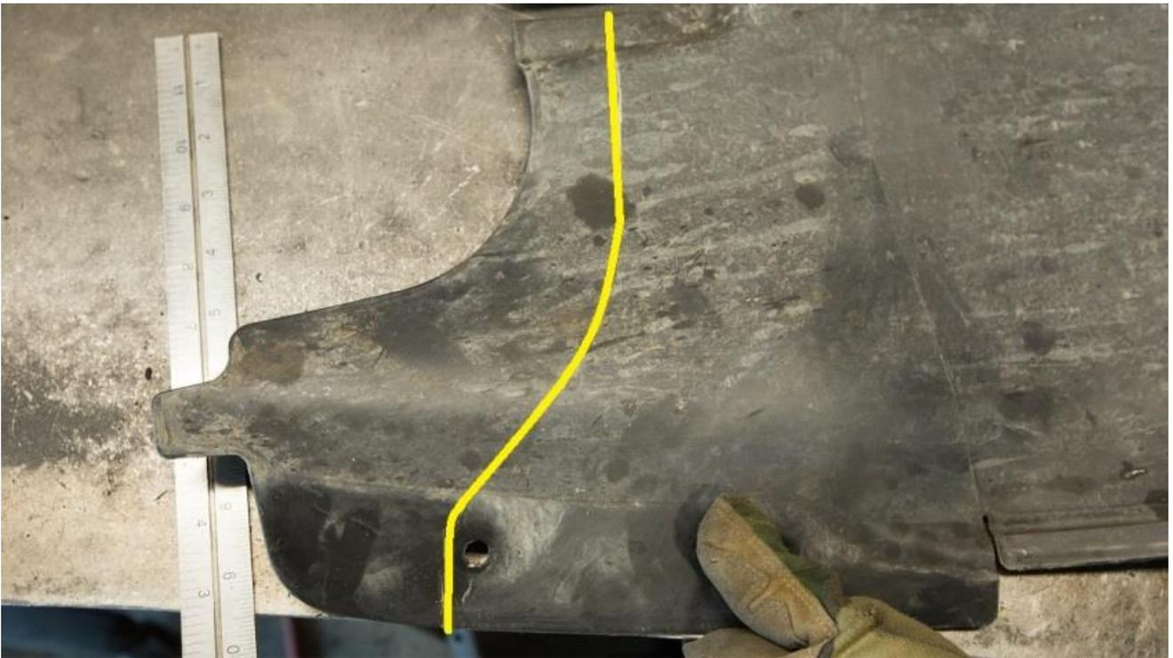
81) Re-install the fender well liners in the reverse order of removal. The trimmed liners should appear as shown below.
