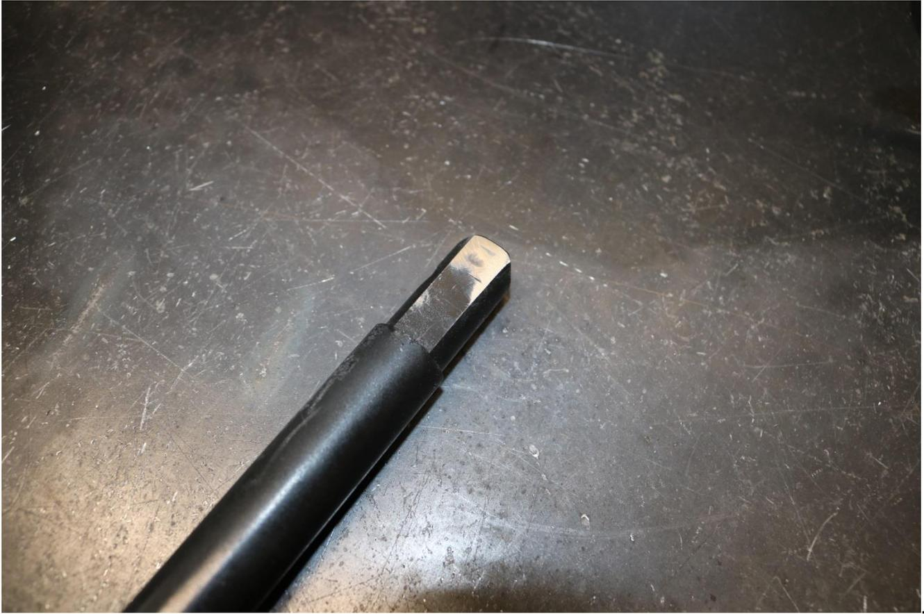
88) Test fit the steering shaft extension onto the steering shaft as shown below.
