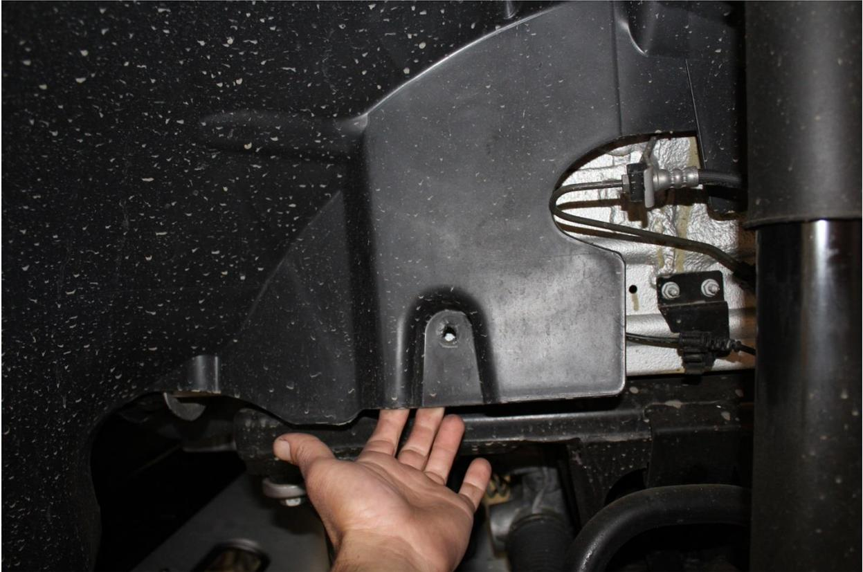
27) Next pull the inner fender well liner away from the bumper and out from under the fender lip until it appears as shown.
