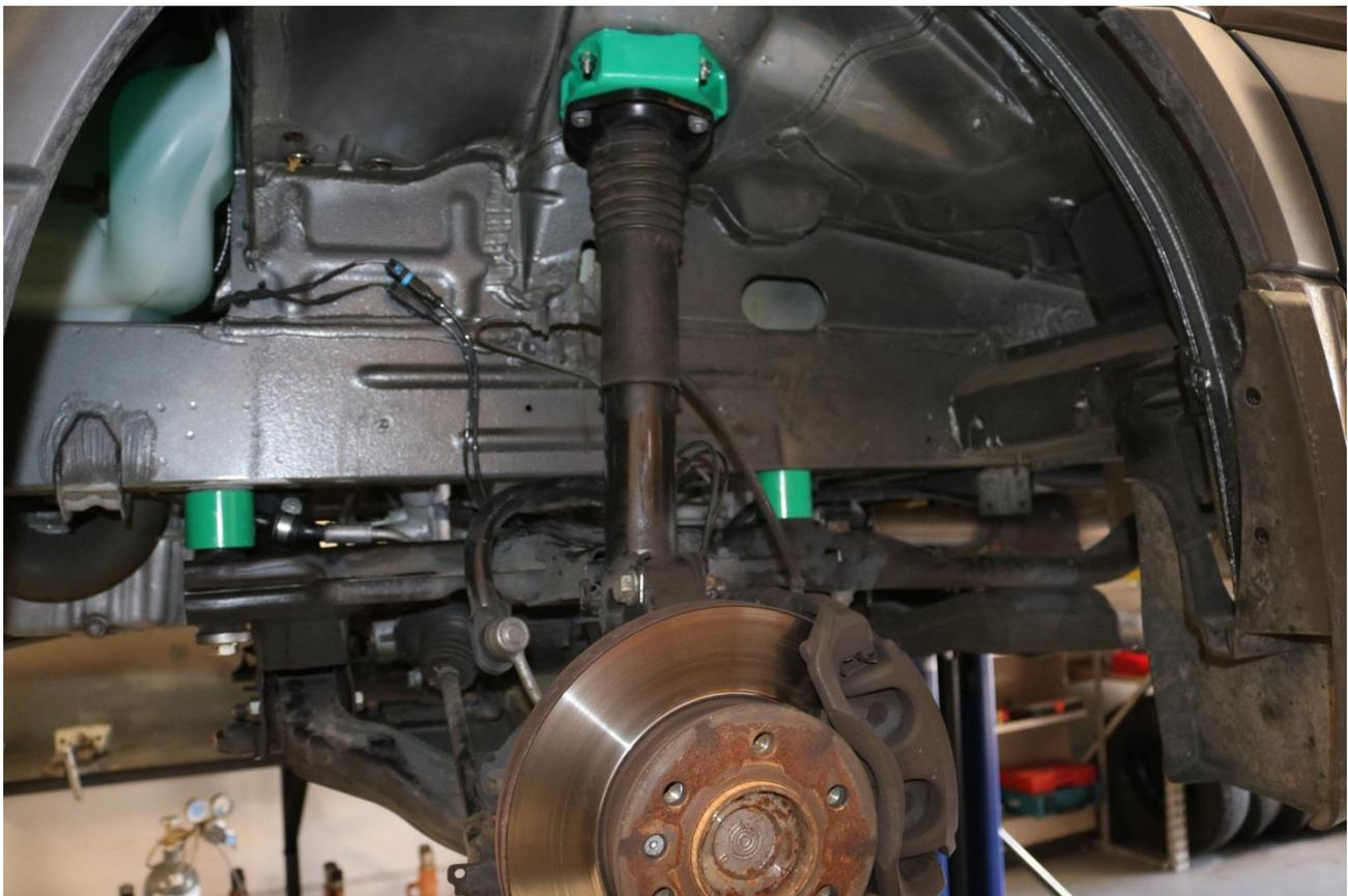
69) Torque lower strut bolts to 127 ft-lbs (172 N.m).
