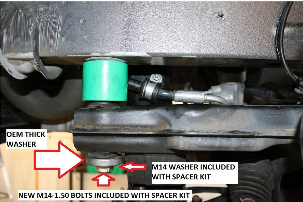
49) Snug all 6 bolts but do not torque at this time. Final torquing will occur once the motor mount spacers are installed and the engine / transmission support jacks & jack stands can be removed.
