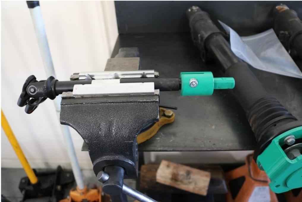
91) Install the steering shaft onto the splines of the rack and pinion. Be careful not to damage the plastic alignment tab on the splines. Once fitted, install the T-45 torx bolt removed in step 9. Again, we recommend using a dab of blue Loctite on the threads. Torque the bolt to 18 ft-lbs (24N.m)
