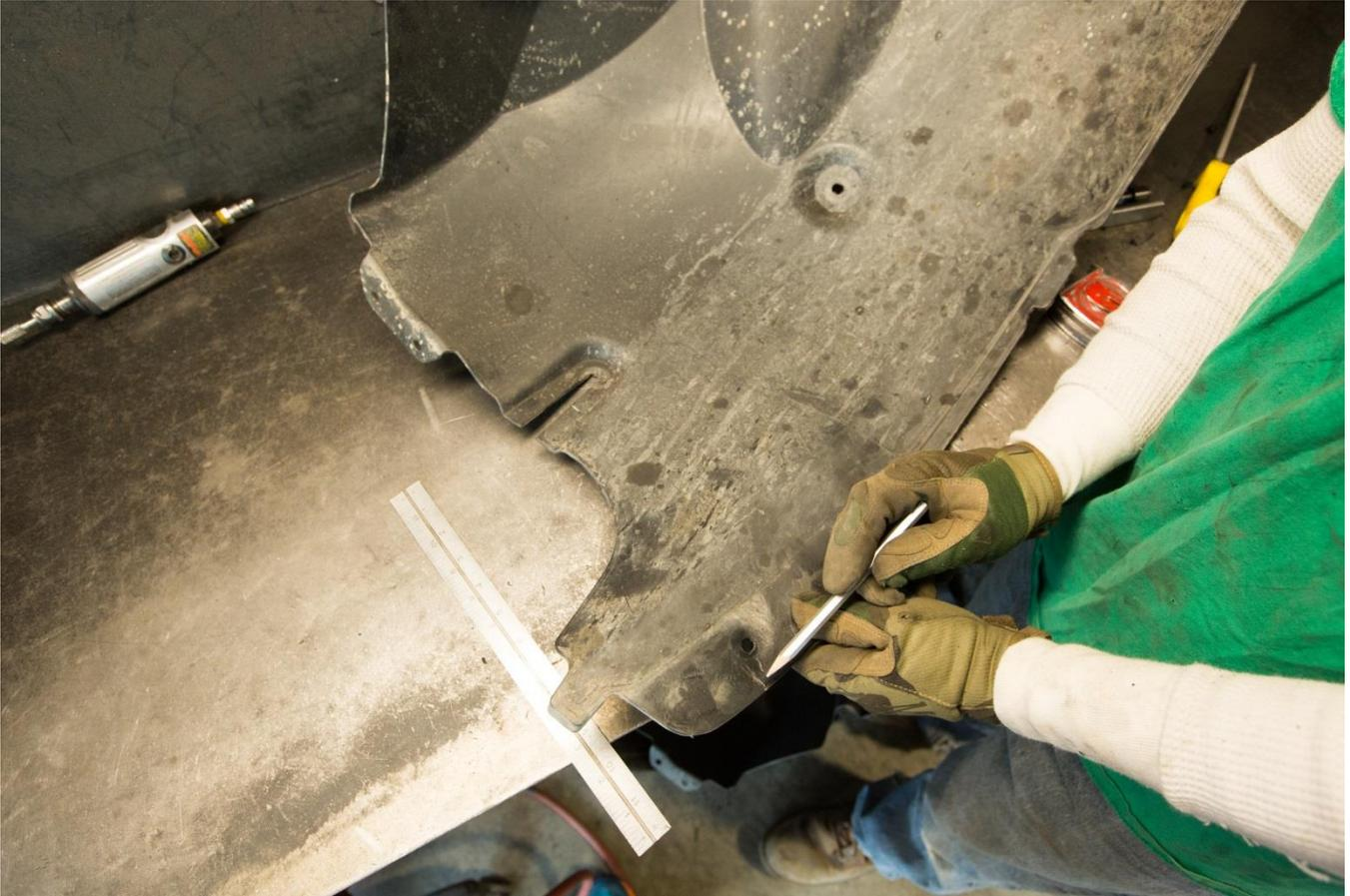
80) Connect the marked lines as shown and trim on the line.
