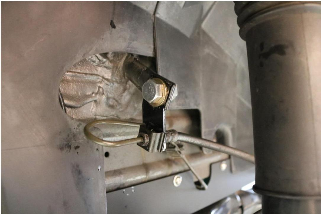
96) Orient the tab as shown above. Tighten the M12 bolt to 50 ft-lbs (67 N.m). Reconnect the hard line to the brake hose and snug the brake line fitting tight.
