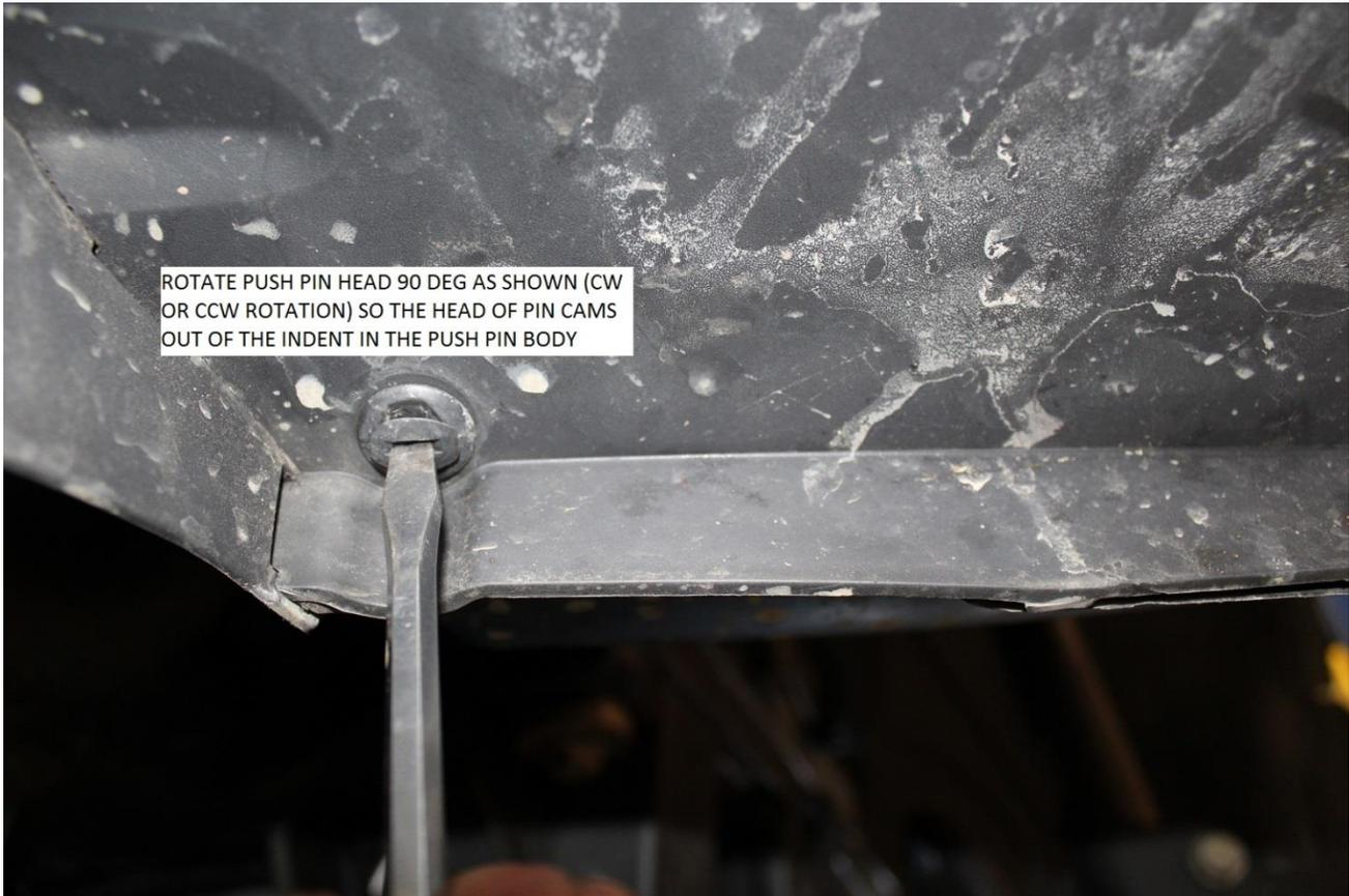
ROTATE PUSH PIN HEAD 90 DEG AS SHOWN (CW OR CCW ROTATION) SO THE HEAD OF PIN CAMS OUT OF THE INDENT IN THE PUSH PIN BODY
