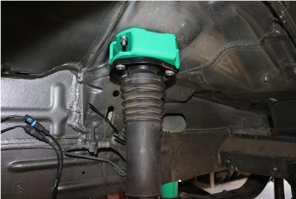
67) With all bolts installed and snug, torque to 21 ft-lbs (28 N.m)
