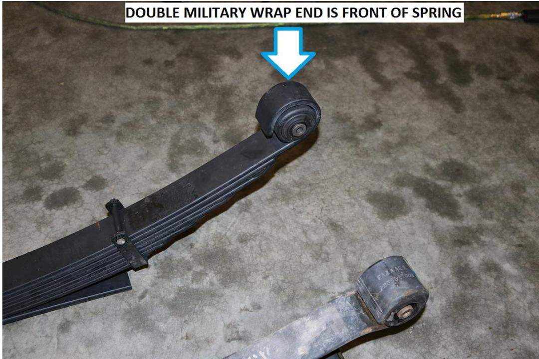
11) Install the leaf springs into the vehicle. We have found it easiest to install the springs upside down and then rotating them up into position once under the vehicle.
