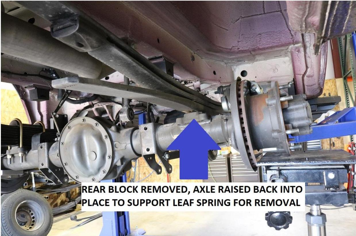
**REAR BLOCK REMOVED, AXLE RAISED BACK INTO PLACE TO SUPPORT LEAF SPRING FOR REMOVAL**
