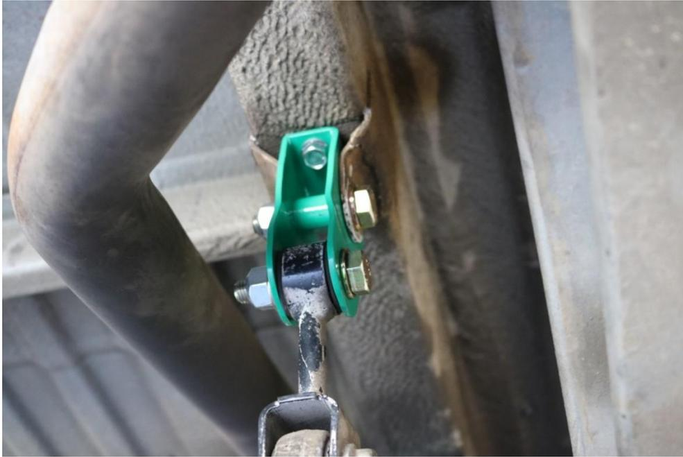
39) Complete rear sway bar installation by securing the sway bar end links to the drop brackets. Use the remaining M12-1.5 x 60mm long bolts provided in the kit with a washer under both the bolt head and stover nut. With a 19mm socket and wrench, torque both upper and lower M12 hardware on the drop bracket to 60 ft-lbs (95 N.m).
