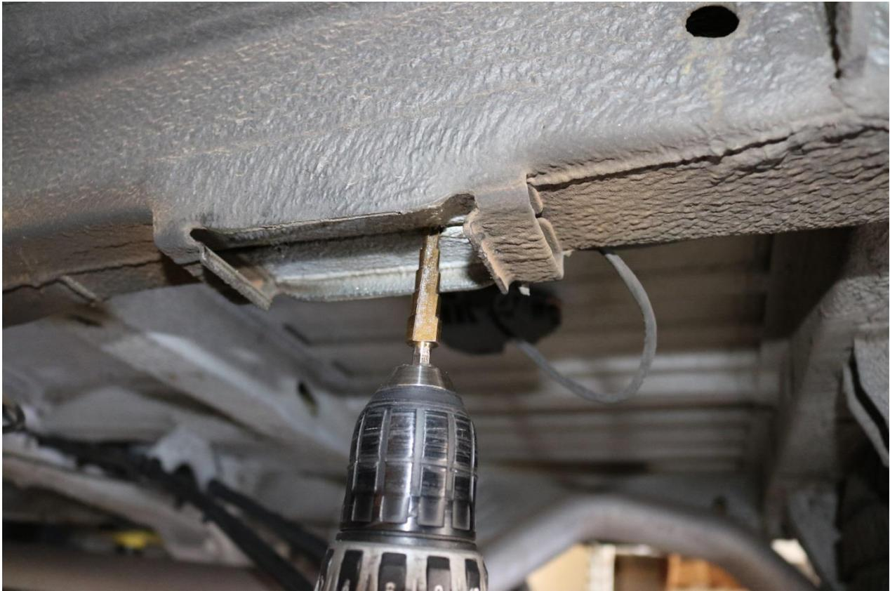
23) With both holes drilled, position the bump stop drop bracket in place and secure it to the chassis using the 5/16-18 x 1" long thread cutting screws included with the kit. Use a nut driver or drill with a 1/4" bit adapter and a 1/2" socket to install the screw. Try to keep the drill / driver as straight as possible when cutting the threads.
