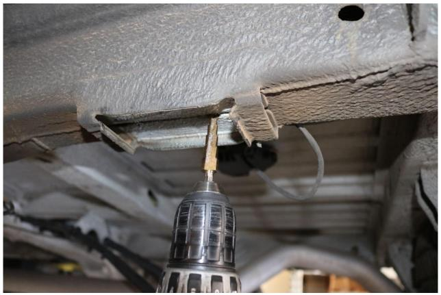
23) With both holes drilled, positions the bump stop drop bracket in place and secure it to the chassis using the 5/16-18 x 1" long thread cutting screws included with the kit. Use a nut driver or drill with a ¼" bit adapter and a ½" socket to install the screw. Try to keep the drill / driver as straight as possible when cutting the threads.
