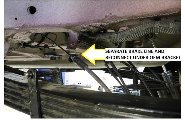
3) Fit the 400801 brake line drop bracket as shown below. Use the M12-1.50 x 25mm long bolt provided with the kit to align the bracket as shown. Mark the top hole and drill using a ¼" (6mm) drill bit.
