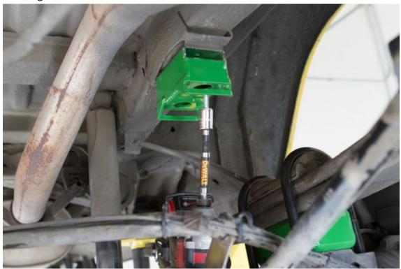
24) Use drill / driver to snug bolts into place. Do not fully tighten using drill / driver. Torque bolts to 13 ftlbs (17 N.m). 25) With drop brackets installed and hardware torqued to spec, thoroughly coat the rubber bump stops with Windex or a similar glass cleaner.
