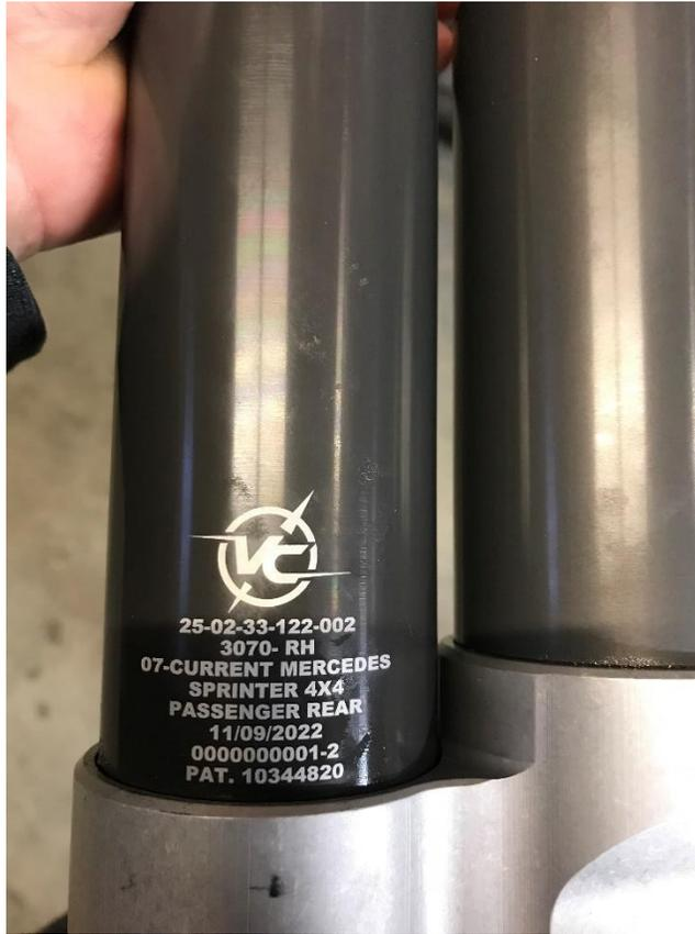
5) The SP2 must be set prior to fitting the shock to the van. Adjust the SP2 mode adjust by rotating the shaft 360 degrees in the direction as specified below for the corresponding van weights:
