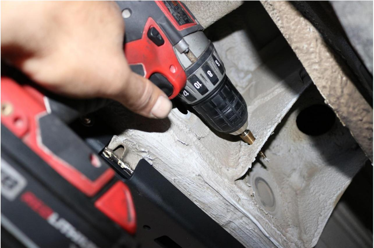
30) Once the hole is drilled touch up any exposed areas of metal with a quality paint to prevent corrosion and re-install the bracket. Start all hardware before tightening.
