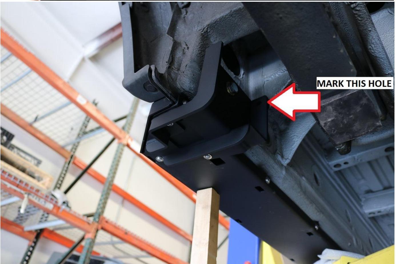
28) Snug all the attachment bolts and mark the front gusset hole on the body as referenced above.
