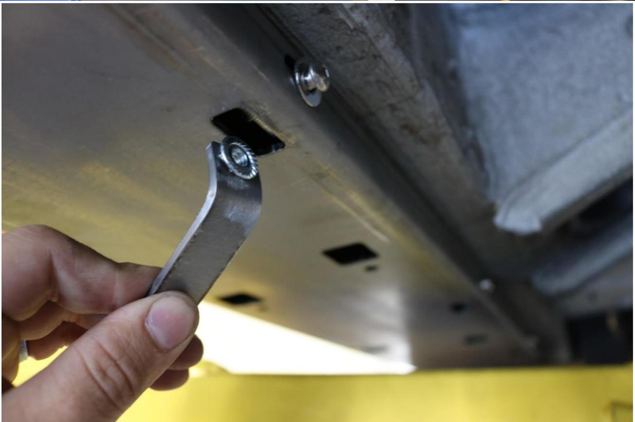
13) Once all inner and outer bolts have been installed with their respective flange nuts on the inside.
