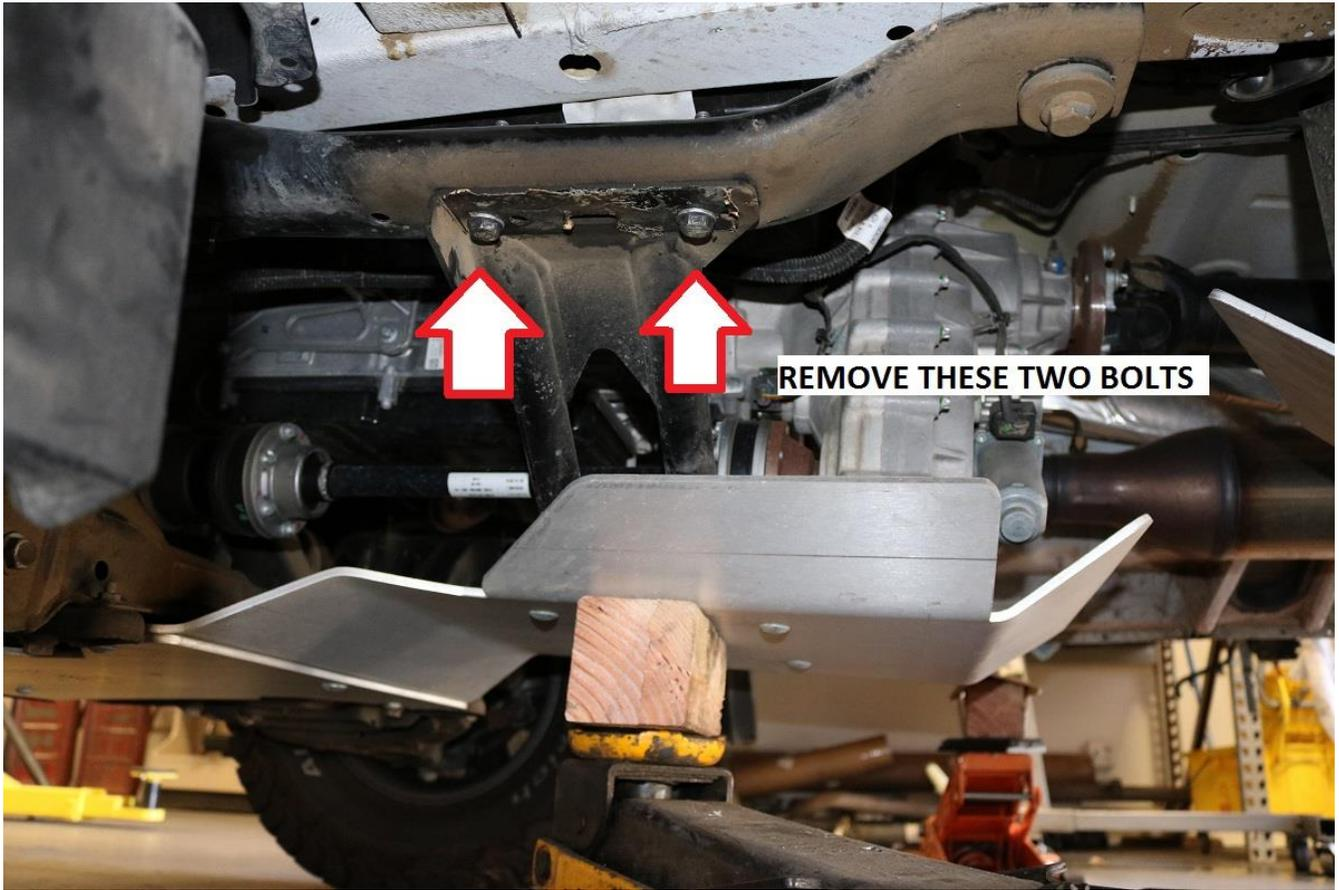
17) Install the 4022-03 Front Chassis Tie-in on the vehicle. These tie-in brackets are left and right specific and will only go on one way. Note image below for reference, showing the orientation of the bracket for the left side (driver side) of the vehicle.
