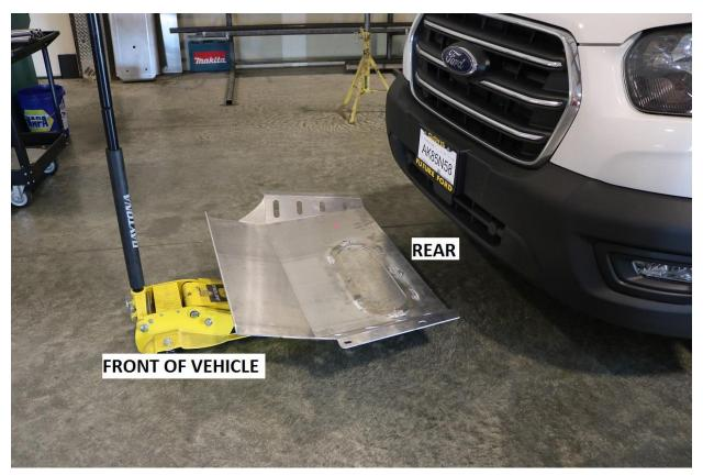
7) Fit the skid plate to the bumper support bars as shown using the ½-13 hardware included in the kit. Use a washer under both the bolt head and the nut. Start and snug all 4 bolts using a ¾" socket / wrench.
