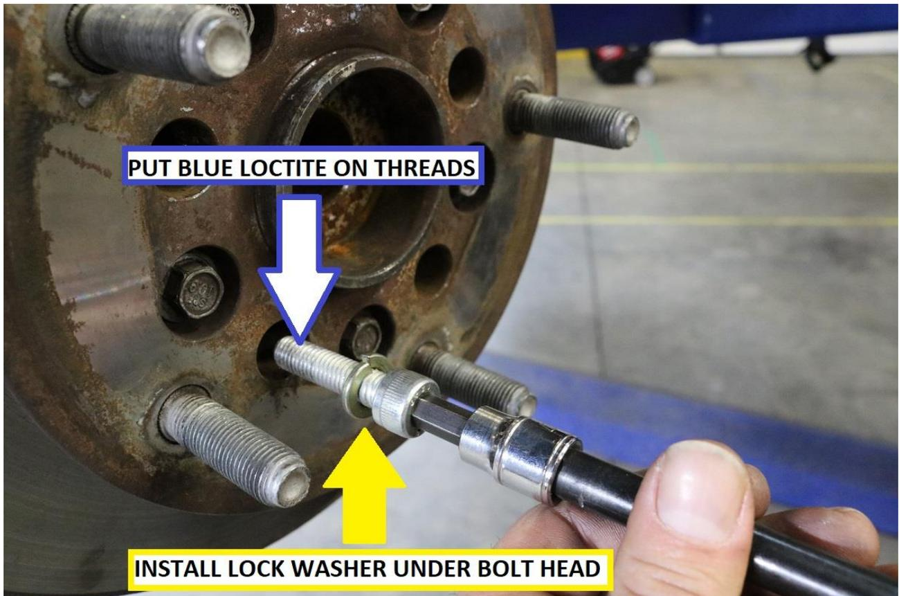
24) Reconnect the sway bar end link to the strut.
