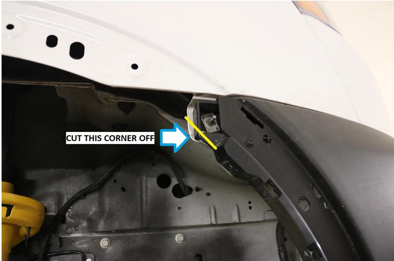
29) Lastly, the front bottom corner of the plastic front bumper fascia needs to be trimmed slightly for tire clearance.
