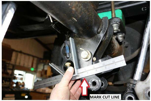
10) Remove the M14 bolt and bracket from the vehicle and cut on the marked line from the previous step. Use a 4-1/2" angle grinder with metal cut off wheel or similar cutting tool. Deburr any sharp or rough edges after cutting with a flap disc or similar metal sanding tool.
