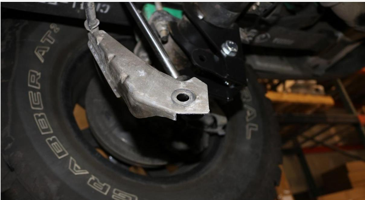
**FINISHED CUT BRACKET SHOULD APPEAR AS SHOWN - AGAIN BE SURE TO PAINT ANY EXPOSED AREAS OF METAL AT THIS TIME**
