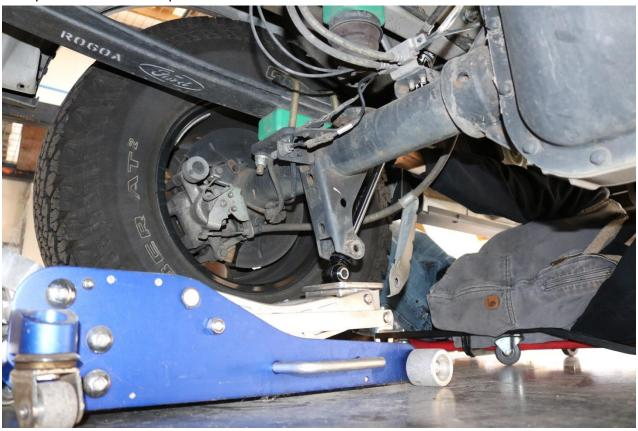
7) Install the OEM lower shock bolt from the outside so the nut is towards the inside of the vehicle.
