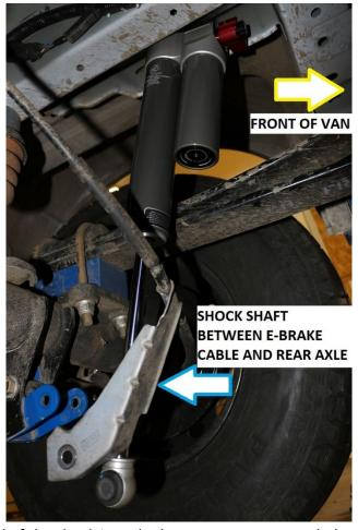
6) Install the opposite end of the shock into the lower mount. Have a helper operate a floor jack to compress the shock into place.
