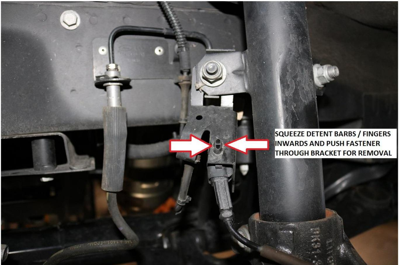
8) Completely remove the wheel speed sensor wiring from the strut. Separate the wheel speed sensor from the chassis harness. See image below for reference.
