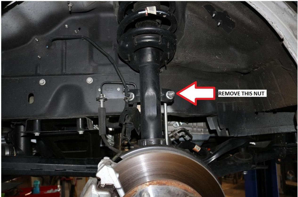
7) Remove the wheel speed sensor wiring from the strut. See image below for reference.
