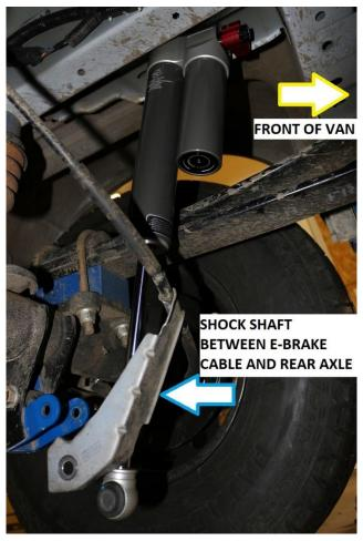
7) With the top of the shock bolted into the upper mount, ensure the shock shaft is extended out all the way. Adjust the SP2 mode adjust by rotating the shaft 360 degrees in the direction as specified below for the corresponding van weights:
