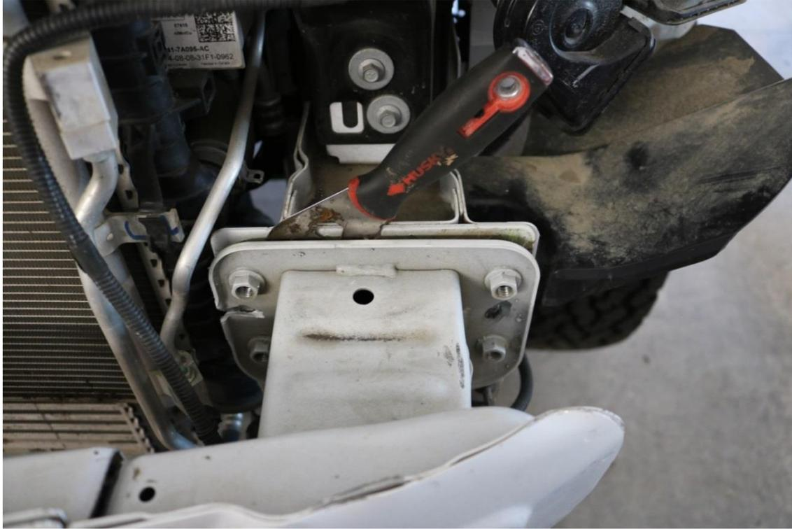
24) With the front bumper removed, remove the lower front bumper valence. Locate the four 13mm bolts on each side and remove.
