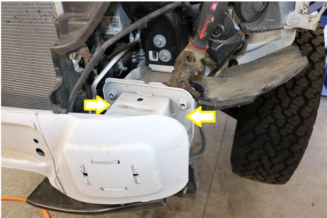
23) Once the spot welds have been located, grind / cut them out.
