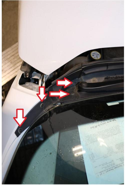
3) Loosen or fully remove the 4 screws in the center of the push-pin fastener with a Phillips screwdriver or powered nut driver. With the screws loosened or fully removed, remove the remaining portion of the push pin fastener using an automotive trim removal tool. See image below for reference.
