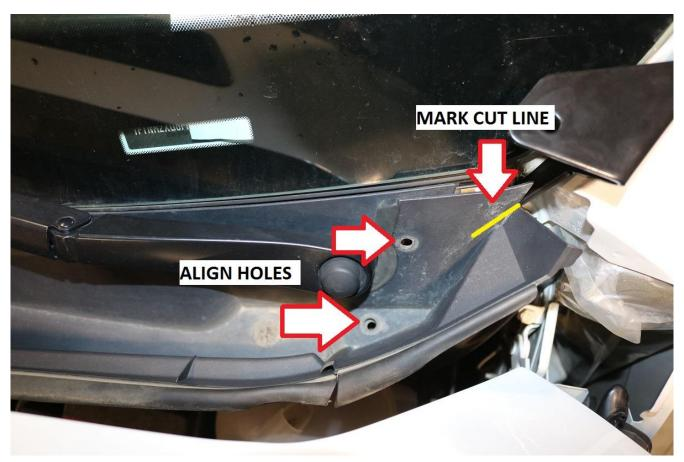
12) Cut a slot on the marked line. Use a 3" cut off wheel or dremel or similar tool that will easily cut through plastic. The slot only needs to be about 1/8" wide and approximately 1" long. Test fit the trim piece and continue trimming as necessary. The finished trim piece should appear as shown below.
