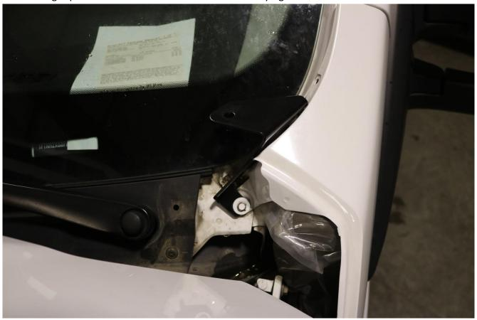
8) Install the included M6-1.00 x 30MM long stainless flat head bolt into the upper mounting hole. Use a 4mm allen wrench for installation.
