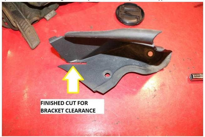
13) Once satisfied with the cut, deburr any rough or sharp edges and install the trim piece back onto the vehicle using the plastic screw push pin fittings removed in step 3.
