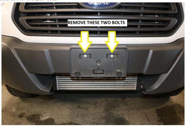
8) Remove the two bumper plugs using a small flat blade screwdriver.
