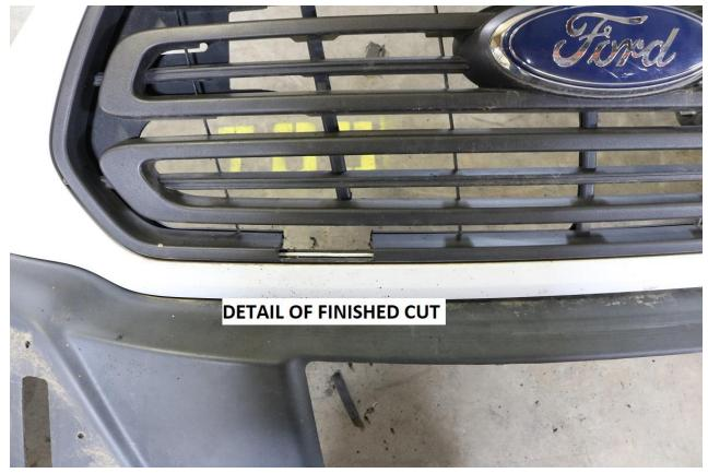
28) Test fit the trimmed grill to ensure it clears the light mount tabs. If everything clears, re-install the bumper / grill in the reverse order of removal.
