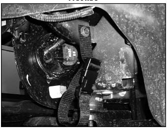
Note: The links must be completely removed from the vehicle when sway bar is disconnected and stowed in the vehicle with the retaining pins and spacers. Swing the sway bar up so that it is LEVEL and retain with straps. Do not drive the vehicle on-road with the sway bar disconnected.
