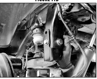
14. Reinstall the track bar bracket with the 9/16" hardware (BP 748) along with the provided crush sleeve (48) inside the factory mount. Run the bolt through the new bracket, OE mount and sleeve (Fig 12). Leave hardware loose.
