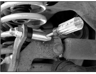
17. Attach the lower studs to the axle with included 1/2" nylock nuts. Tighten to 65 ft-lbs. The shortest stud will go on the Passenger's side, medium length stud goes on the Driver's side (Opposite for RHD vehicles). (Fig 4c, 4d)
