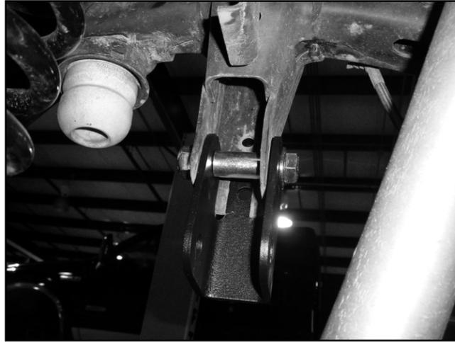
15. Fasten the new bracket to the frame through the outer holes using the provided 7/16" hardware (BP 748). The bottom hole uses the larger diameter USS washer on the inside to go against the slot in the frame. Torque 7/16" hardware to 40 ft-lbs (Fig 13).
