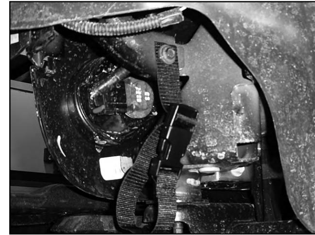
*Note: The links must be completely removed from the vehicle when sway bar is disconnected and stowed in the vehicle with the retaining pins and spacers. Swinging the sway bar up so that it is LEVEL and retain with straps. Do not drive the vehicle on-road with the sway bar disconnected.*
