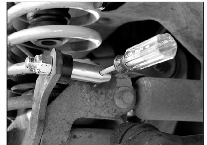
17. Attach the lower studs to the axle with included 1/2" nylock nuts. Tighten to 65 ft-lbs. The shortest stud will go on the Passenger's side, medium length stud goes on the Driver's side (Opposite for RHD vehicles). (Fig 4c, 4d)
