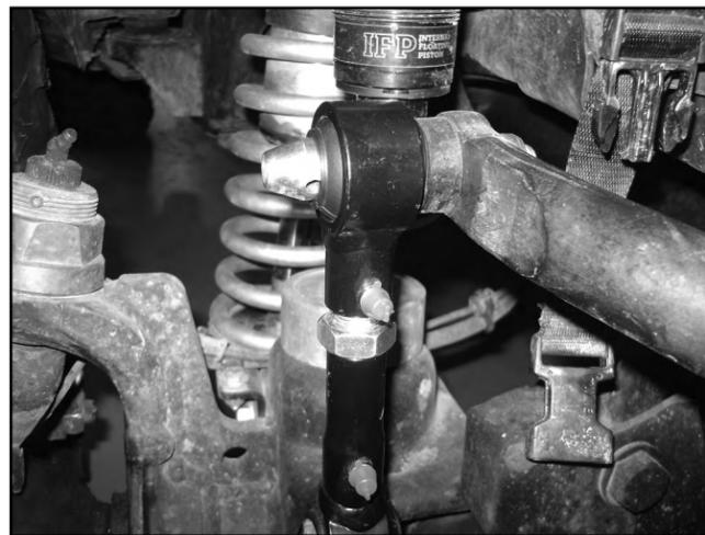
19. Locate the existing inner fender bolt up near the front body mount. Remove the bolt and attach the new lanyard to the inner fender with the bolt. Torque bolt to 10 ft-lbs. Slide the male clip up the lanyard and attach the female clip to it. This will be the stowed position for the lanyard when not in use. Do not wrap around the swap bar when the sway bar is connected.
