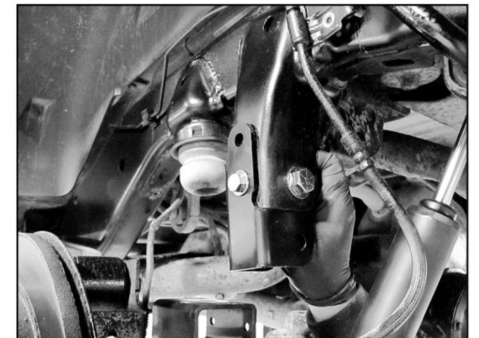
14. Reinstall the track bar bracket with the 9/16" hardware (BP 748) along with the provided crush sleeve (48) inside the factory mount. Run the bolt through the new bracket, OE mount and sleeve (Fig 12). Leave hardware loose.
