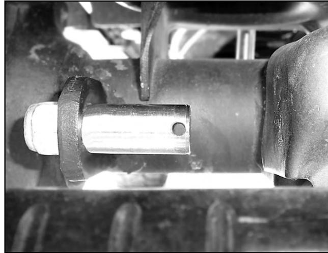
18. Place sway bar links onto pins, secure with click pins as shown. (Fig 4e, 4f)
