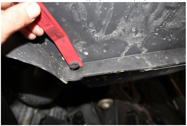
39) Using the same automotive trim removal tool, pry up under the head of the push pin body to fully removal the fastener. Remove these from both sides of the vehicle.
