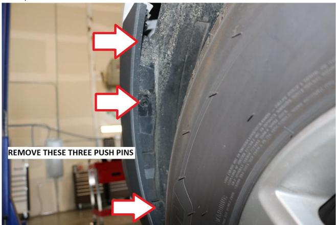
8) Look up from the iniside of the fender where the plastic bumper cover meets the metal fender and locate the last remaining push pin securing the bumper cover to the vehicle.
