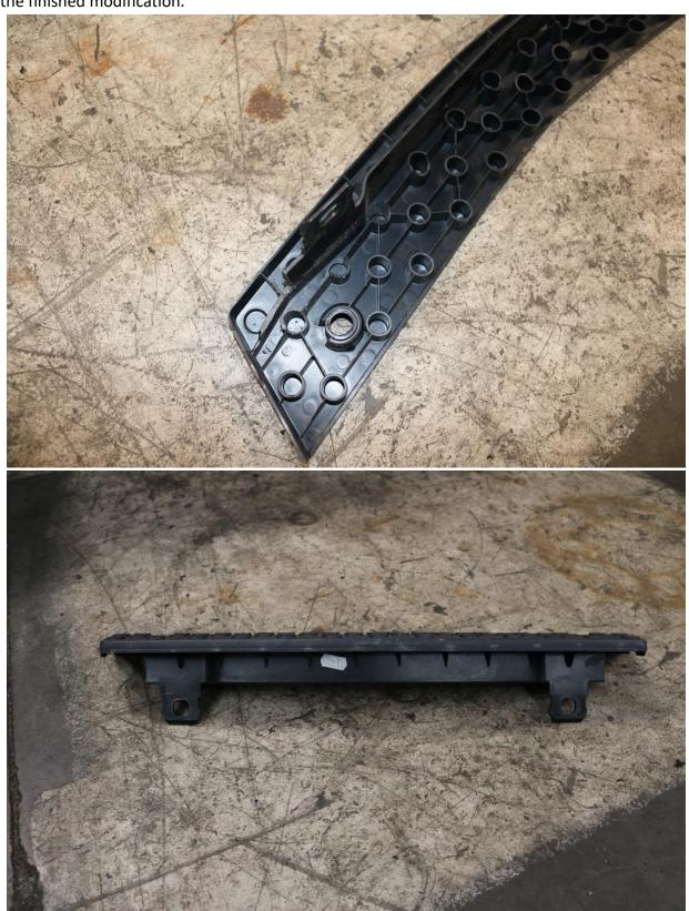
70) Check fit the step tread plate on the front hitch to make sure the holes line up properly in the hitch.
