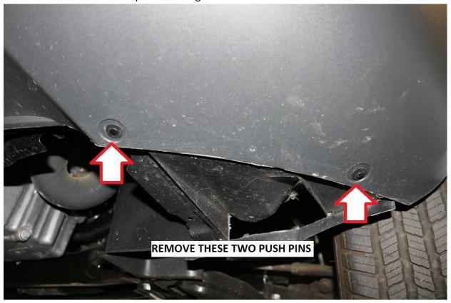
6) Use an automotive trim removal tool to pry up under the head of the push pin prior to prying under the body of the fastener to fully remove it.
