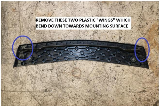
69) Use a small air sander, or angle grinder with sanding disc, or a Dremel style tool to remove these "wings." This will allow the tread plate to sit flat on the front hitch. See images below for reference of the finished modification.
