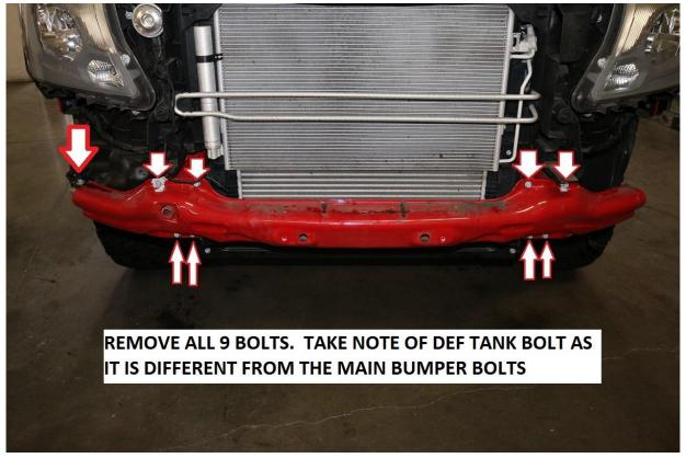
51) Remove bumper from vehicle. Note, some of the glue / undercoating used during assembly can cause the front bumper to be stuck onto the chassis. A rubber mallet or deadblow will help free it from the vehicle.
