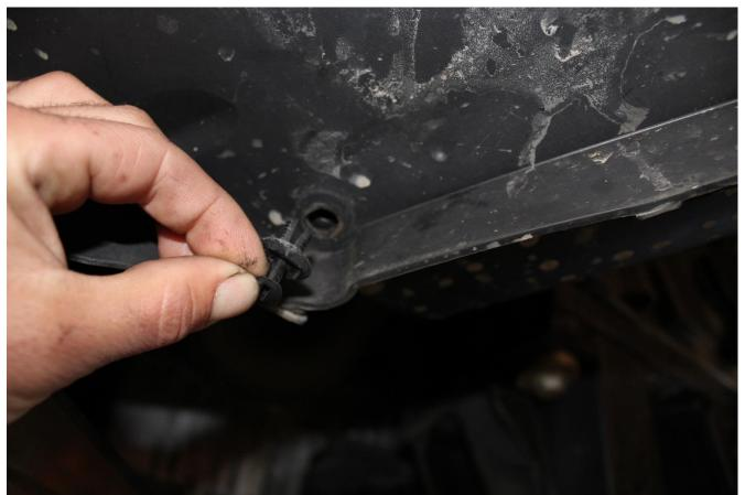
40) Next, on the inside of the fender well, remove the three push pin fasteners near the outer lip of the bumper cover.
