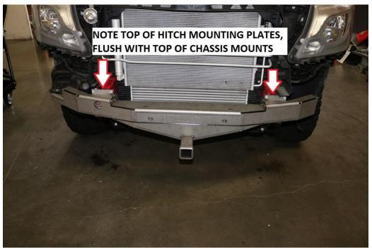
60) Install the included M12-1.50 x 40mm long bolts in replace of the lower over run bolts removed in step 25. Note, it is easier to align the lower DEF tank mounting bolt from by unseating the machined shoulder washer and installing it on the bolt rather than try to align the DEF tank with the winch mount. Be sure to use an included washer under the bolt head. Again, use a dab of blue Loctite on the threads.
