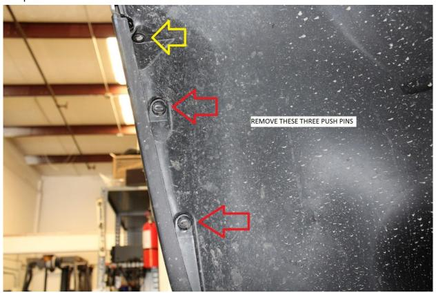
41) Again, make sure to remove these pins on both sides of the vehicle.
