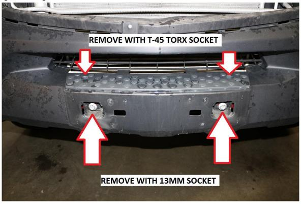
44) At this time the bumper cover is only secured to the vehicle via snap clips where the bumper meets the front fender. Pull the back corner of the bumper cover outwards to separate it from the clips. These clips are fairly tight, so a good strong pull will be needed for separation.
