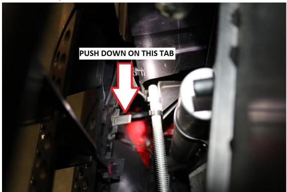
37) Locate the two push pin fasteners located near the front bottom side of the bumper cover which connect the inner fender well liner to the front bumper cover.
