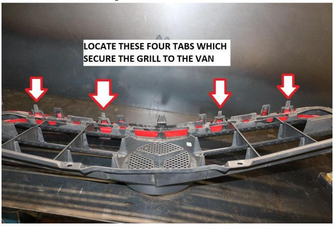
36) Once these tabs are located, push down on them and gently pull the bottom of the grill away from the van and it should easily come free from the vehicle. We have found a long flat nose screwdriver to work well as a tool to push down on the tabs.
