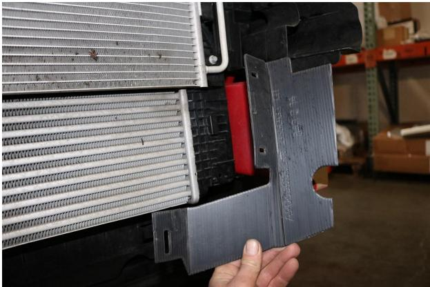
56) A small piece of the intercooler needs to be trimmed for the hitch to fit. See the following two images below for cut reference.
