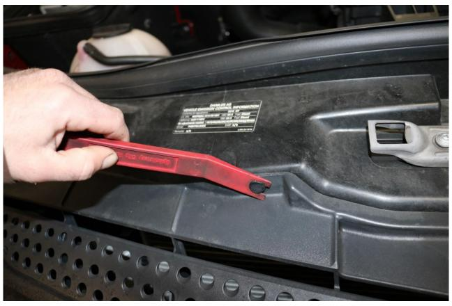
35) With the upper part of the grill separated, gently pull the top of the grill back and locate the four tabs which secure the bottom of the grill to the van.
