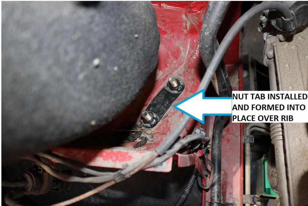
33) Reference steps 22-38 to complete bracket installation on the passenger side. The only real difference between installation on the driver and passenger side is the vertical mounting bolts on the passenger side bracket are both  $\frac{1}{2}$ -13 so a  $\frac{3}{4}$ " wrench is used for both upper bolts.
