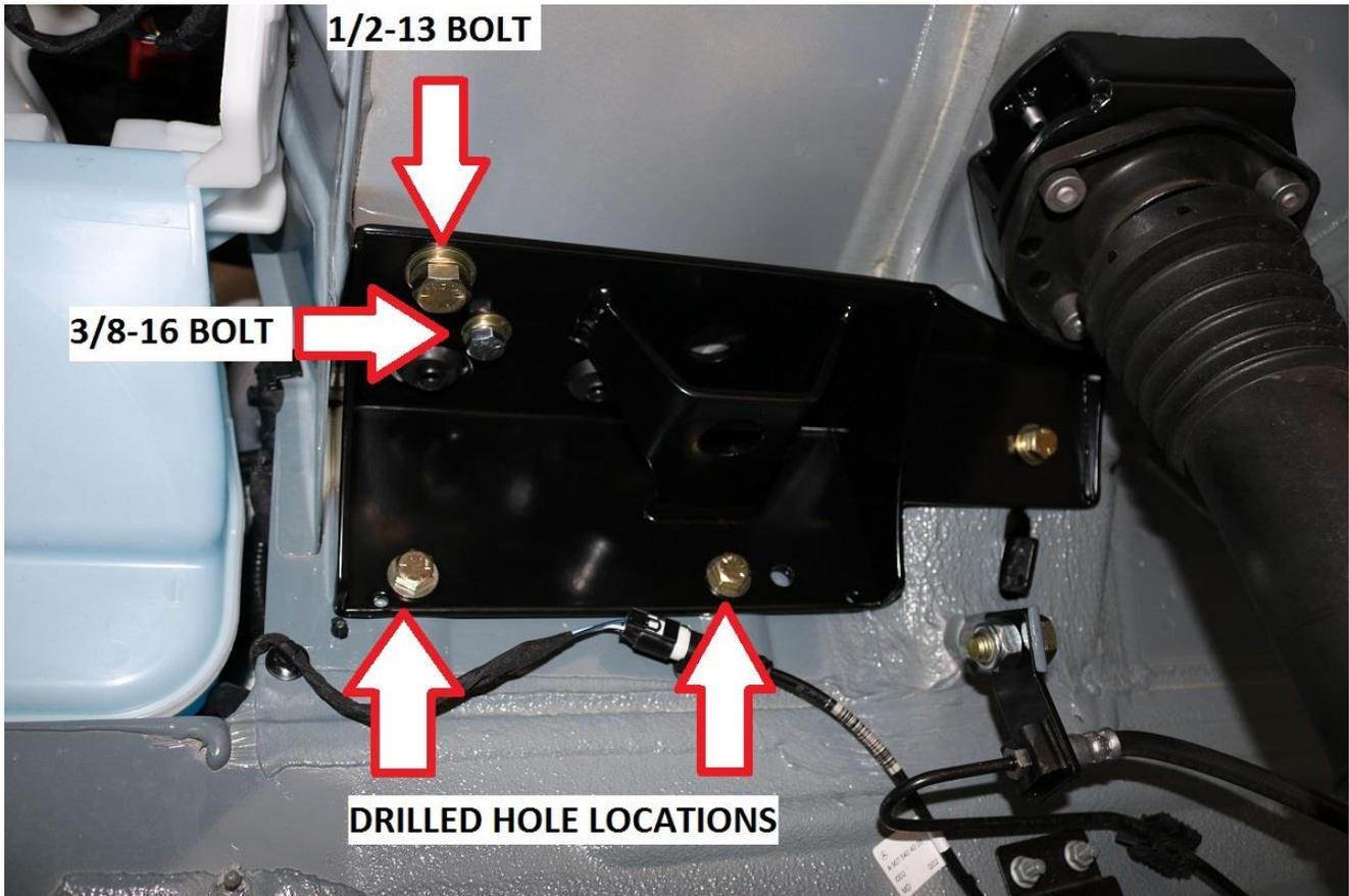
27) With the holes drilled, install the included 3/8-16 x 1" long bolts provided in the kit. Use a washer under the bolt head and under the stover nut on the back side. Snug hardware.
