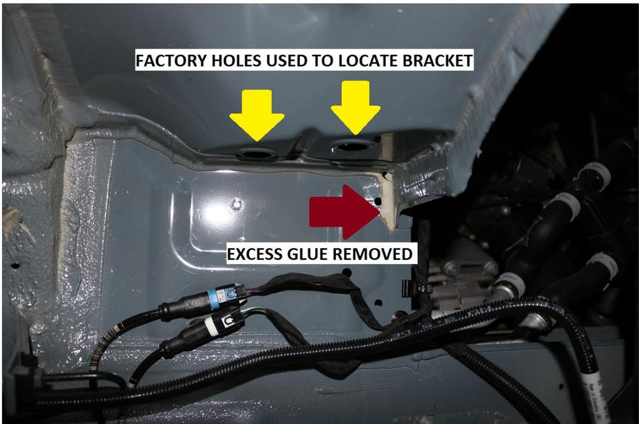
31) Touch up any bare areas of metal with paint to prevent corrosion.
