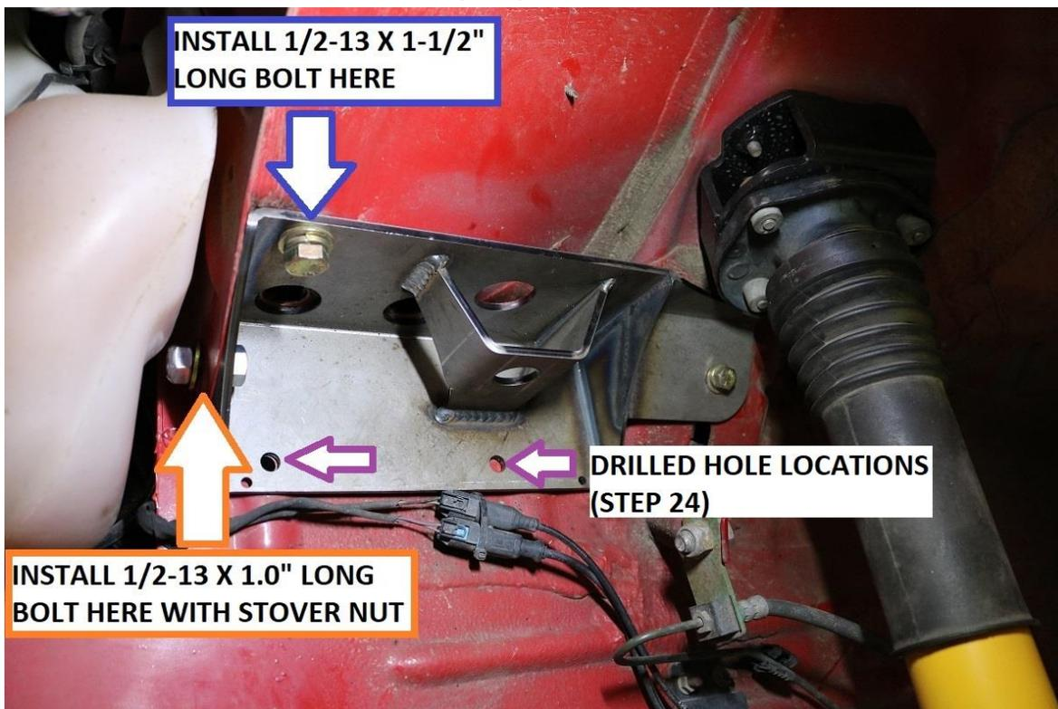
21) Next use the rear nut tab to attach the rear part of the bracket to the chassis.
