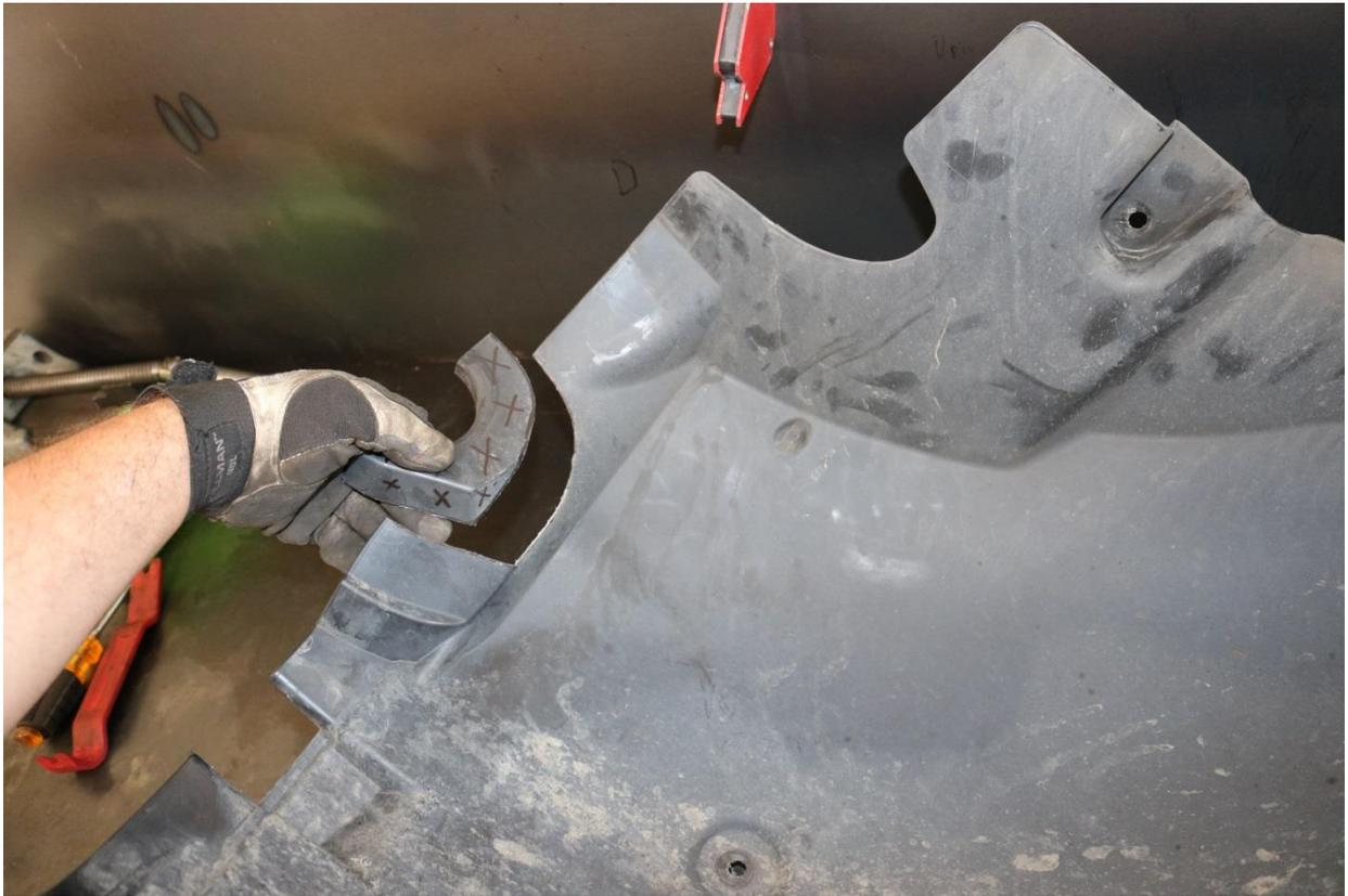
71) The rear half of the fender well liner trimming is very similar. Again, see the images below for reference.
