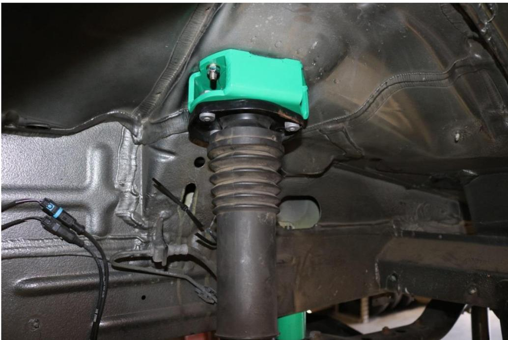
65) With all bolts installed and snug, torque to 21 ft-lbs (28 N.m)
