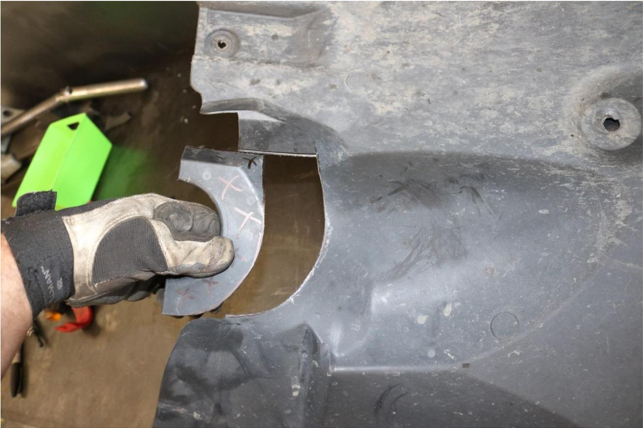
72) Re-install the fender well liners in the reverse order of removal. The trimmed liners should appear as shown below.
