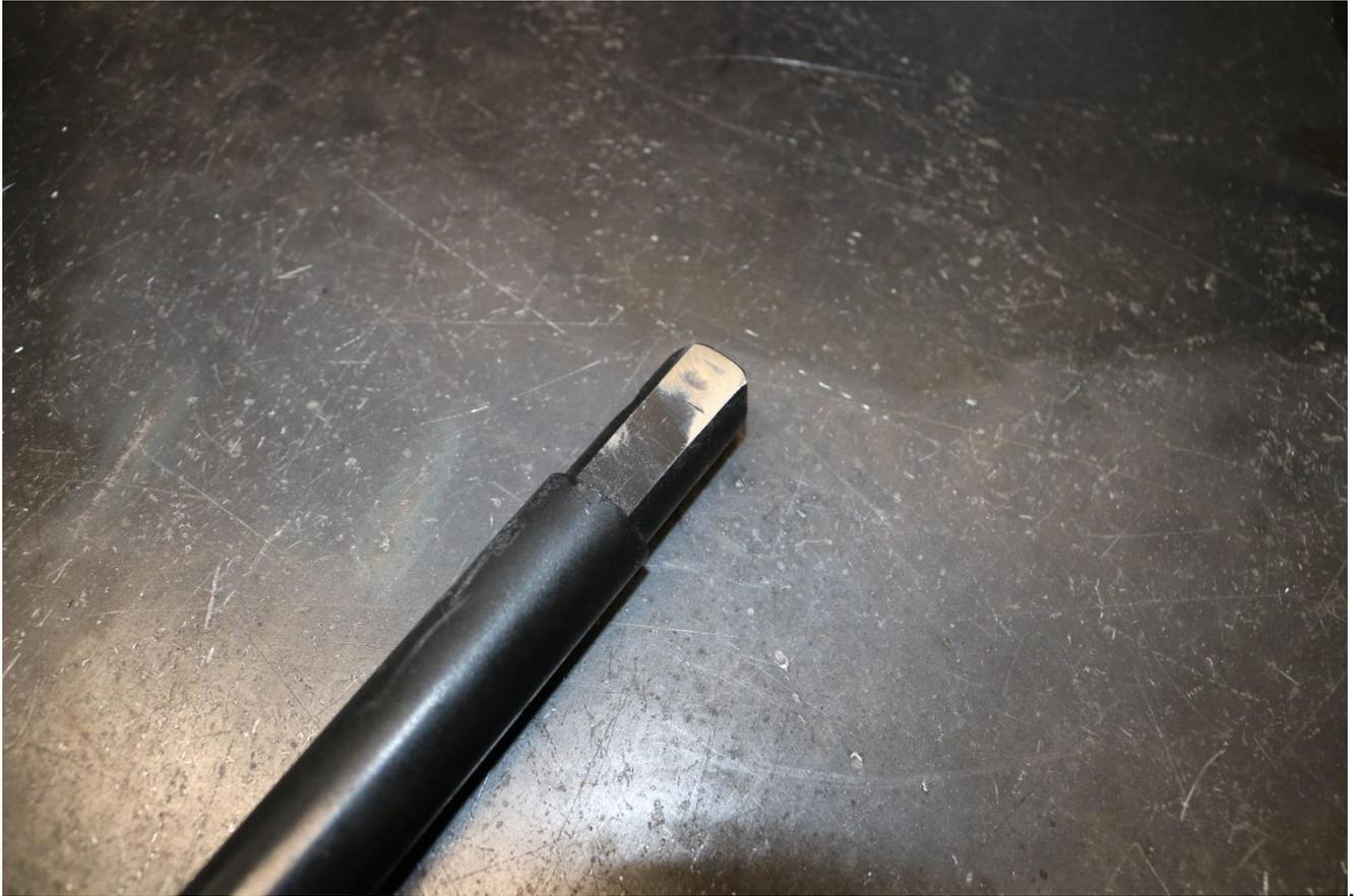
75) Test fit the steering shaft extension onto the steering shaft as shown below.
