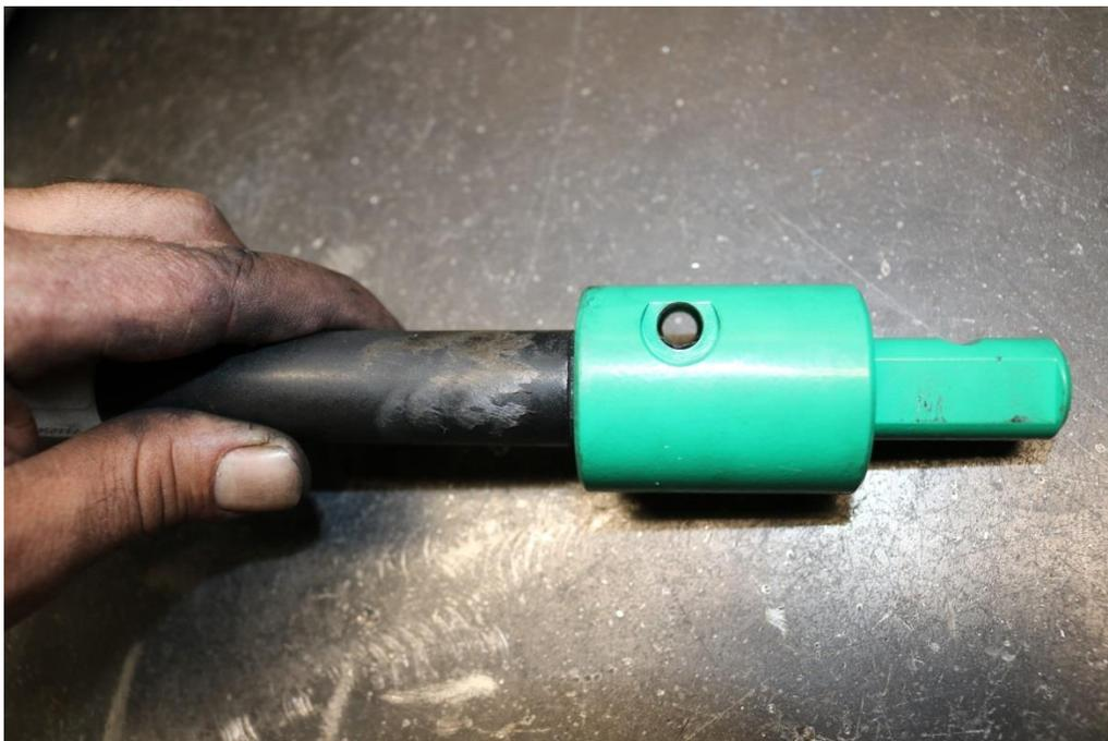
76) If the notch needs to be modified to allow for the bolt to be installed, use a small die grinder with burr bit or a 4-1/2" angle grinder with metal grinding wheel. Remove as little material as possible to allow fitment.
