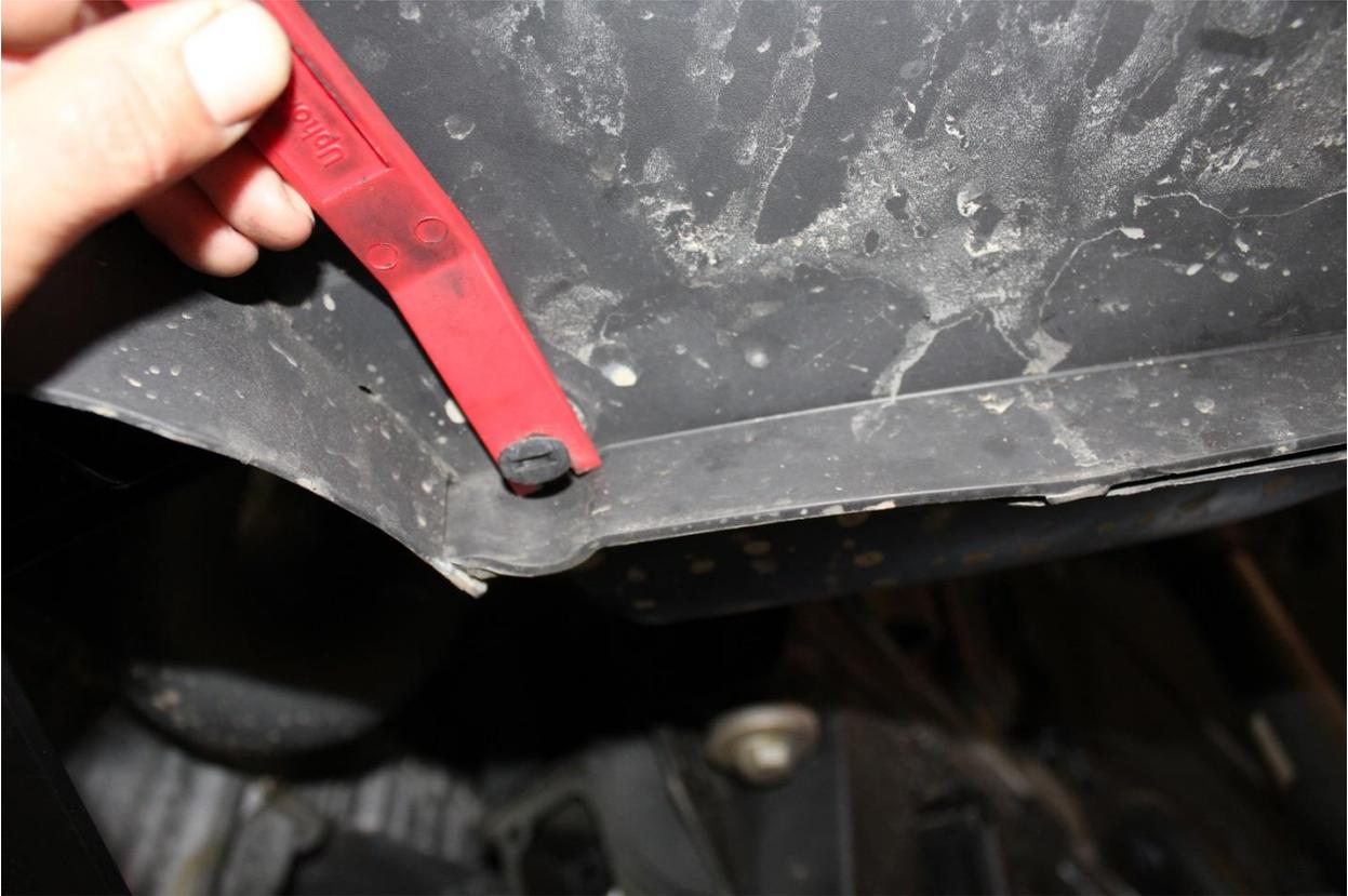
20) Using the same automotive trim removal tool, pry up under the head of the push pin body to fully remove the fastener.
