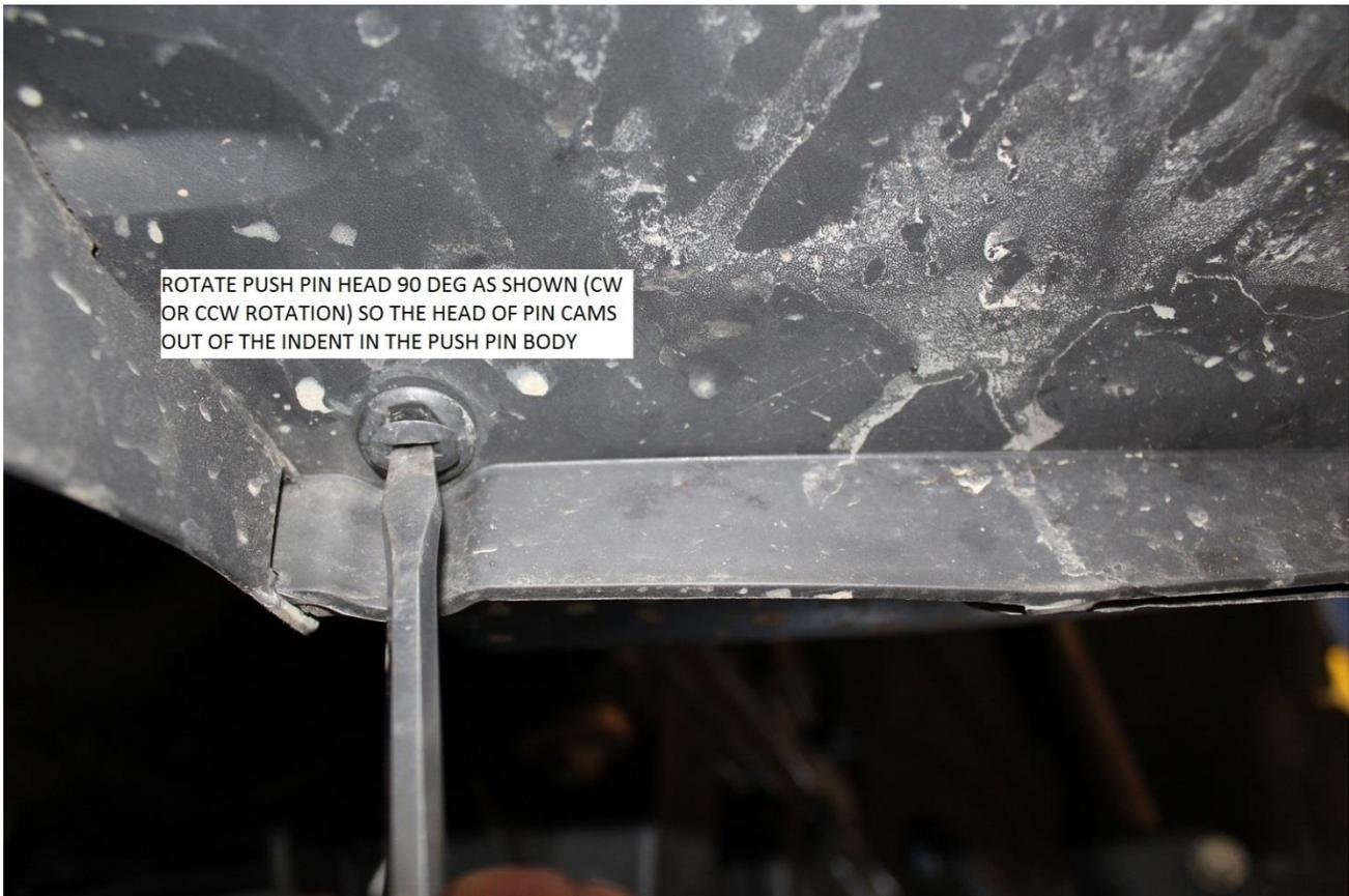
19) Next, using an automotive trim removal tool, pull up the head of the push pin.
