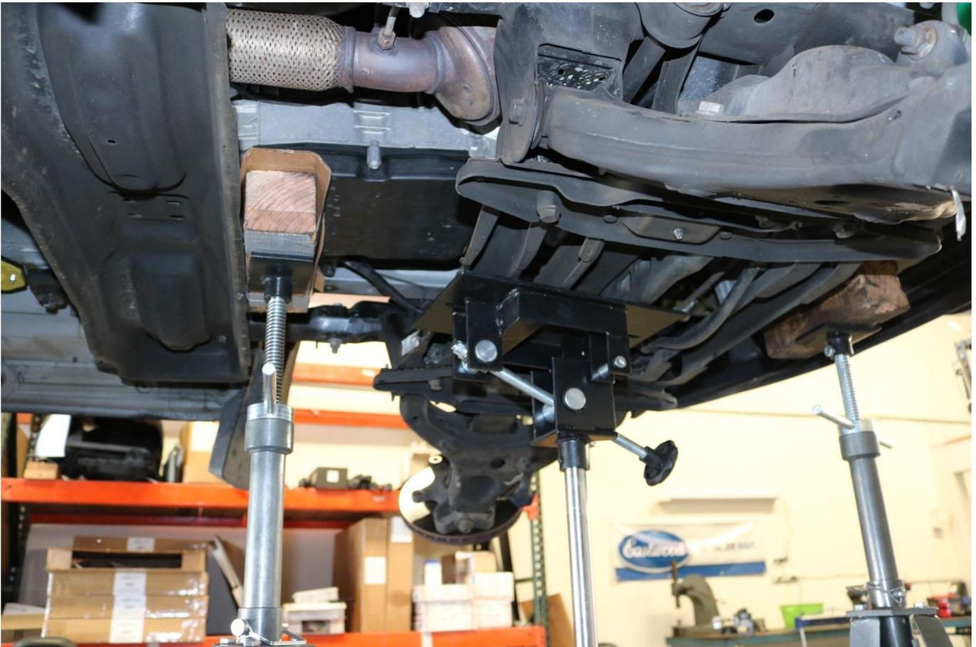
41) The ABS / ESP wiring barb retention clip may need to be pried out of the sub frame for installation of the spacers. Use an automotive trim removal tool to separate the clip from the sub frame.
