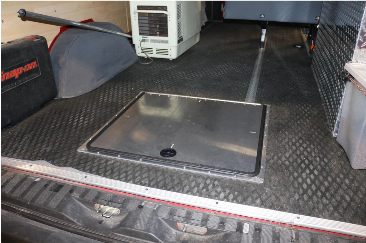
22) Test close the lid with the edge trim installed and ensure the latch grabs the catch in the box and does not have too much up and down play. Adjust the catch up / down as needed for proper lid fitment.
