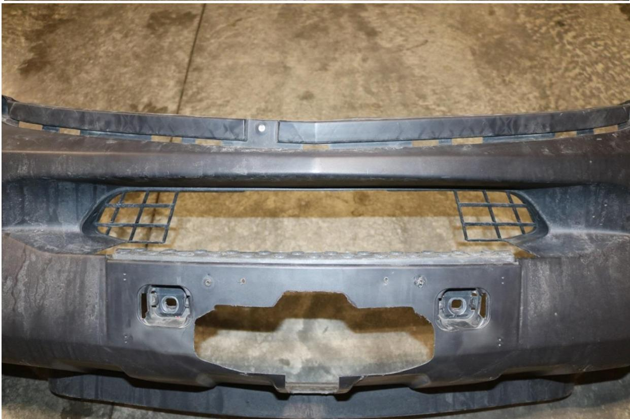
44) If the front receiver is not being installed, trimming of the front bumper cover is now complete and the installer can move along to step 43.
