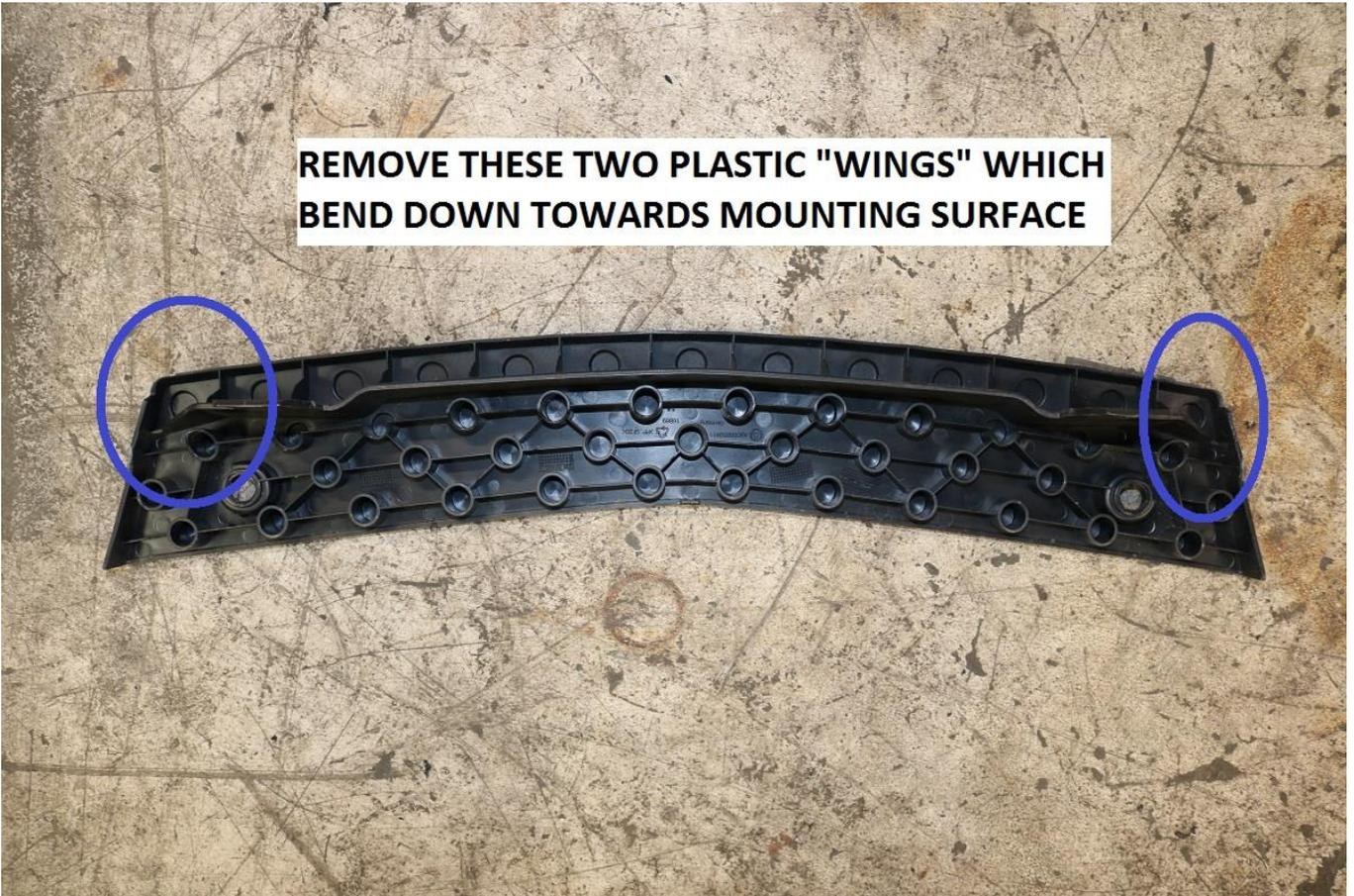
47) Use a small air sander, or angle grinder with sanding disc, or a Dremel style tool to remove these "wings." This will allow the tread plate to sit flat on the front winch mount. See images below for reference of the finished modification.
