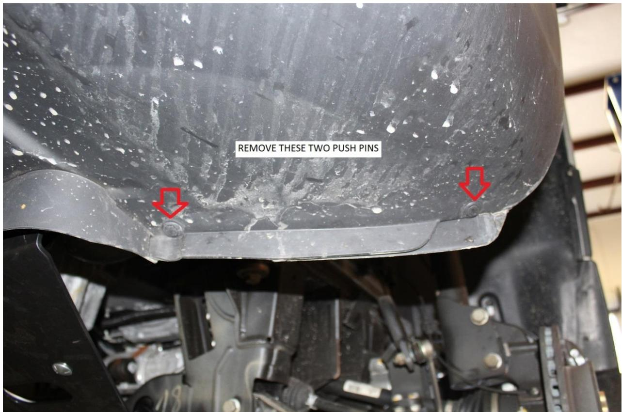
6) This style of push pin is a 2 step removal process.
