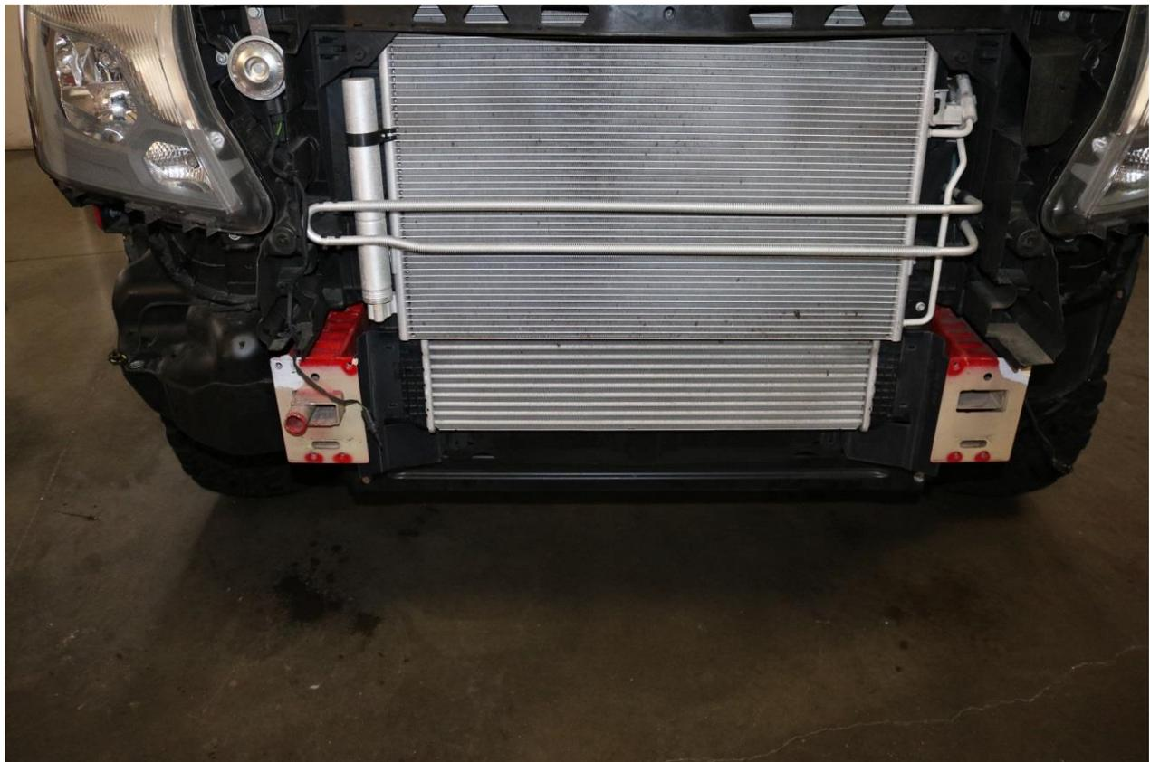
20) Using a metal cutting tool to cut the factory tow point tube flush with the rectangular mounting tube in the chassis. We recommend a 4-1/2" angle grinder with cut off wheel, but a sawzall or similar cutting tool can be used alternatively.
