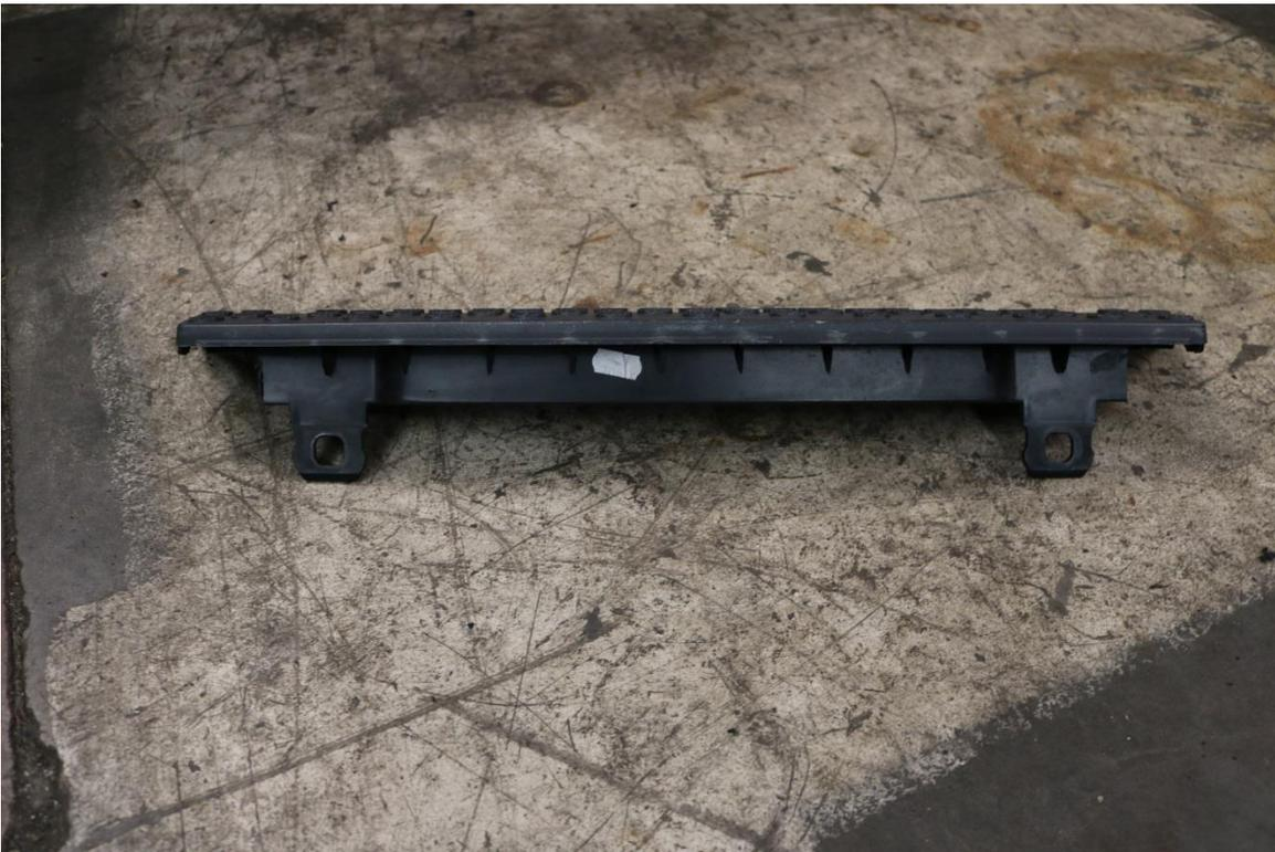
48) Mark a cut line halfway through the tread plate using the raised circular protrusions and the photo below as a guide. Note that the front portion of the tread plate is what will be retained and re-installed onto the vehicle.
