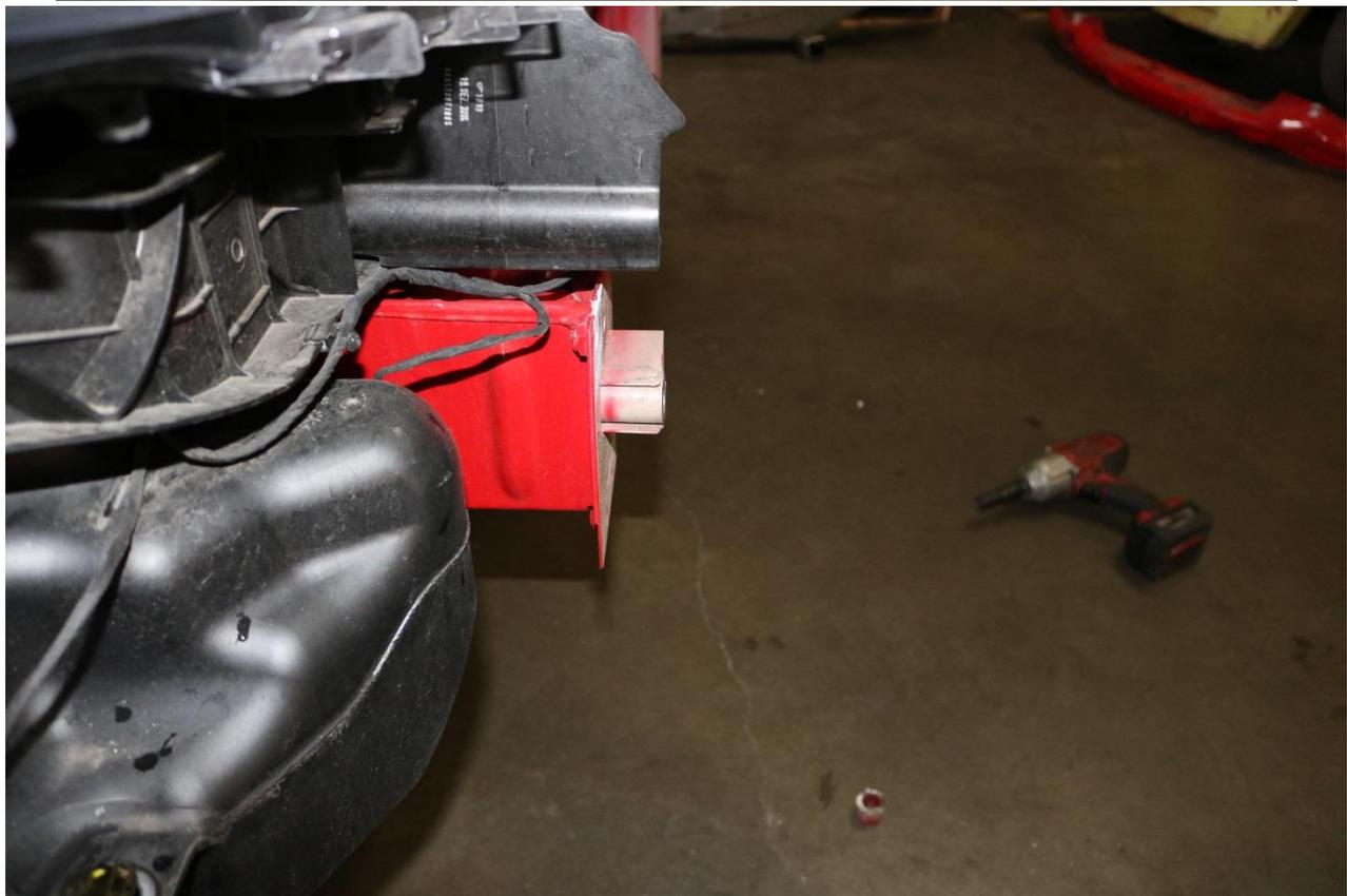
21) Next, on the inside edge of the rectangular protrusion of the factory tow point, mark a diagonal cut line  $\frac{1}{2}$ " (13mm) back and  $\frac{1}{2}$ " outwards and cut the inner corner piece off the rectangular mounting tube of the tow point.
