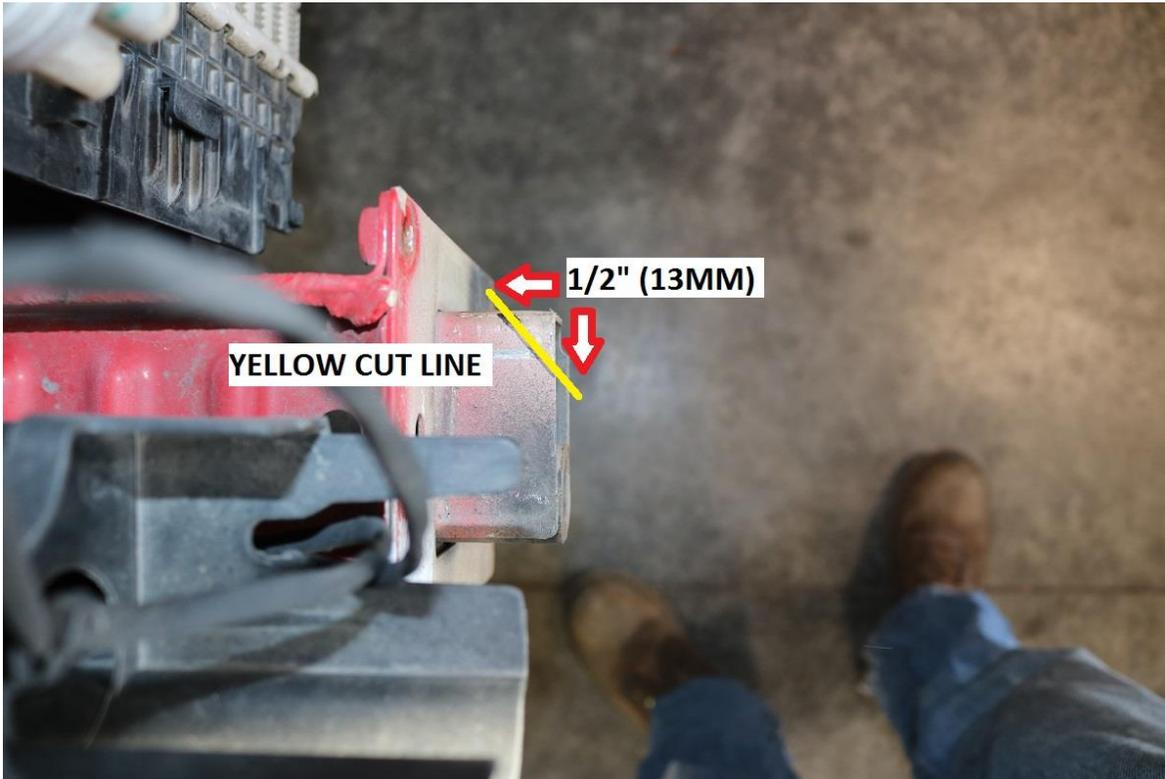
22) After cutting and cleaning up any rough cut edges, paint any exposed areas of bare metal with a quality paint to prevent corrosion.
