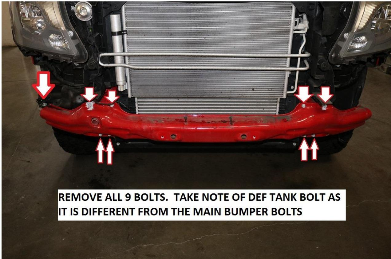
**REMOVE ALL 9 BOLTS. TAKE NOTE OF DEF TANK BOLT AS IT IS DIFFERENT FROM THE MAIN BUMPER BOLTS**
