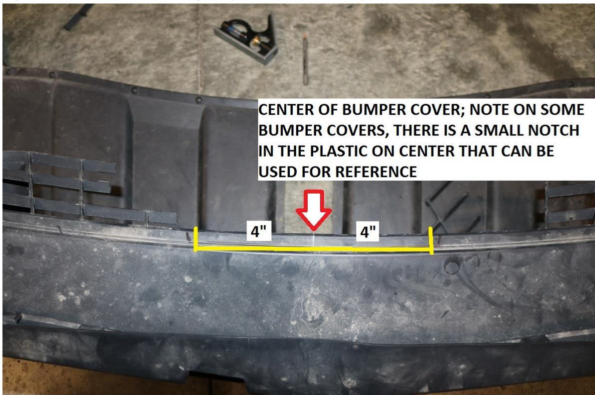
43) Next, fit the fairlead to be used to the bumper cover. Align the bottom of the fairlead with the bottom license plate mounting holes. Trace the outer profile of the fairlead to mark the cutlines.
