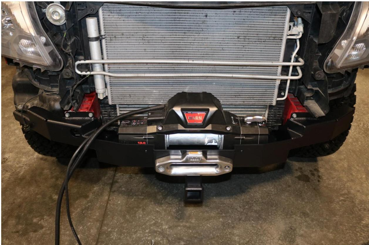
35) Additionally, determine if the shackle points recovery points will be fitted to the vehicle. Steps 35-37 will cover installation of shackle recovery points as well as bumper trimming. If shackle recovery points are not being installed, proceed to step 38
