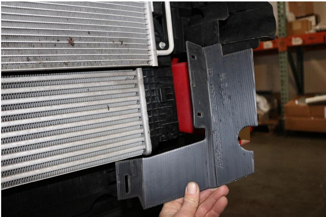
24) A small piece of the intercooler needs to be trimmed for the winch mount to fit. See the following two images below for cut reference.
