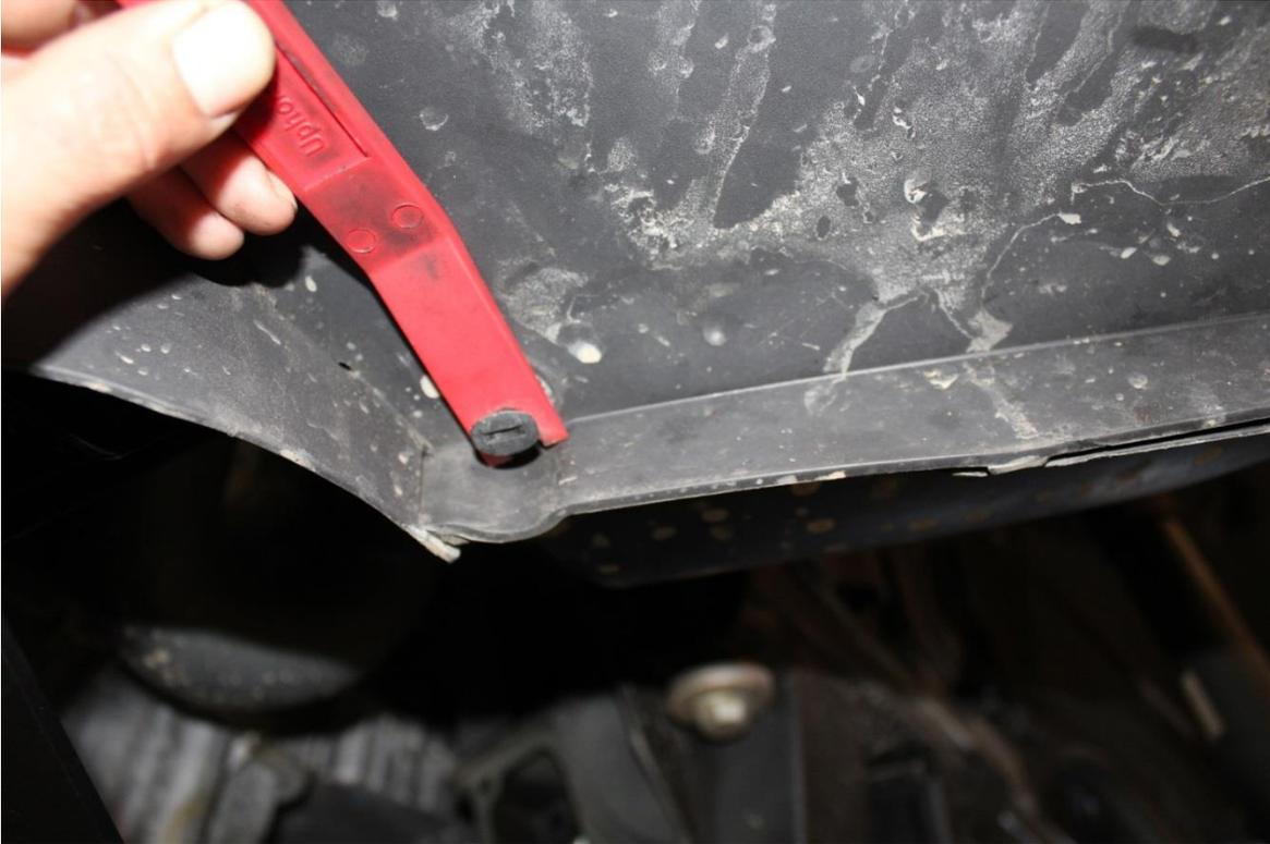
7) Using the same automotive trim removal tool, pry up under the head of the push pin body to fully remove the fastener. Remove these from both sides of the vehicle.
