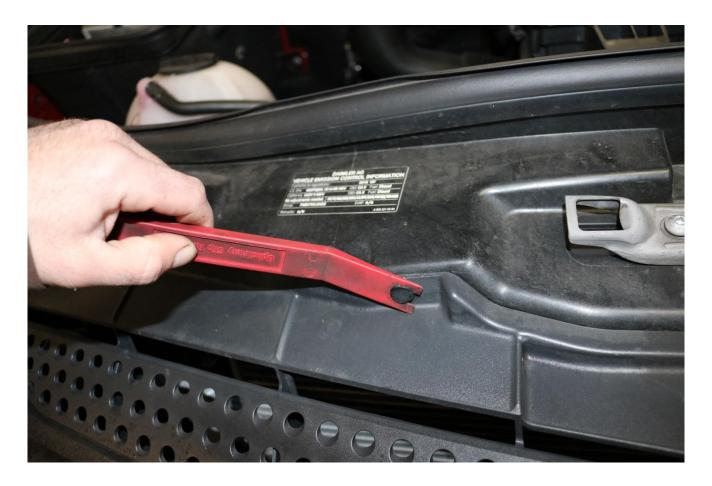
5) With the upper part of the grill separated, gently pull the top of the grill back and locate the four tabs which secure the bottom of the grill to the van.
