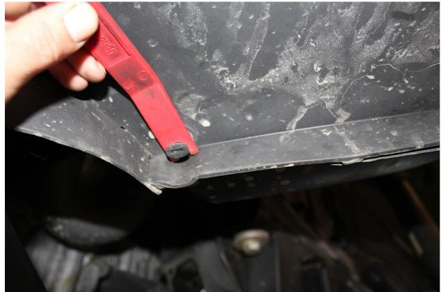
9) Using the same automotive trim removal tool, pry up under the head of the push pin body to fully removal the fastener. Remove these from both sides of the vehicle.
