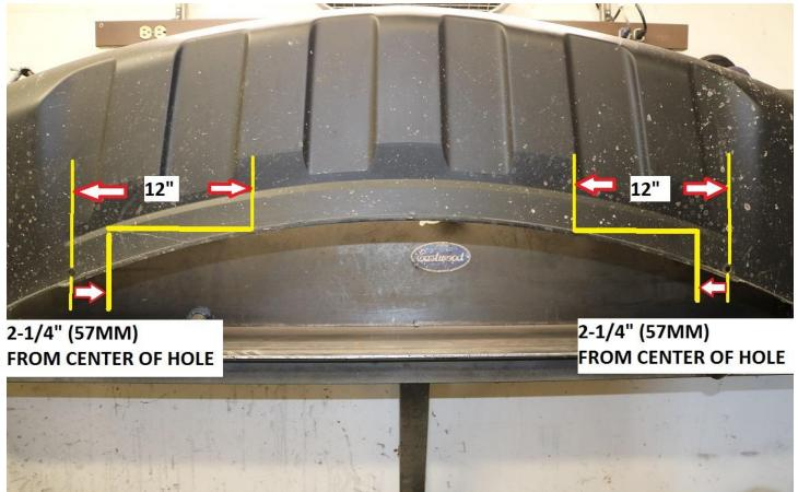
43) Cut on the trim lines and clean up any edges with a file or sander. Finished cut should appear as shown below.
