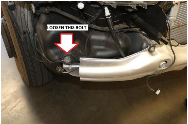
29) On the underside of the vehicle, still on the passenger side, locate the lower mounting bolt for the DEF tank. Remove this bolt using an 18mm socket / wrench. See image below for reference.
