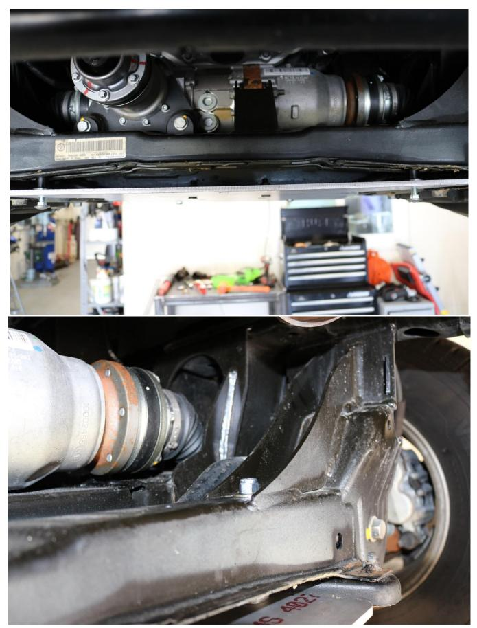
26) Snug all hardware at this time. Snug the flat head socket cap screws first, and then snug all the 3/8" nylock nuts. Use a 9/16" socket or wrench to tighten the carriage bolt hardware.
