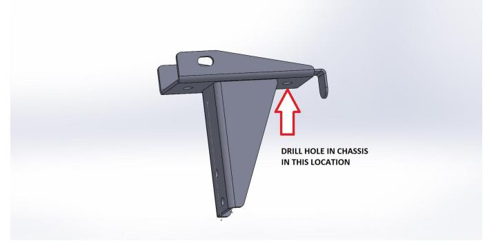
33) Install the included nut tab with the tab pointed downward through the hole in the chassis just behind the overrun bracket. See image below for reference.
