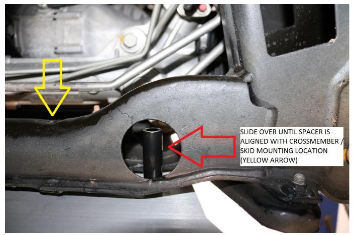
23) Install the 3/8-16 x 3.5" long carriage bolts through the spacer. Use a washer under the nylock nut. Just start the nut. Do not tighten at this time. See image below.
