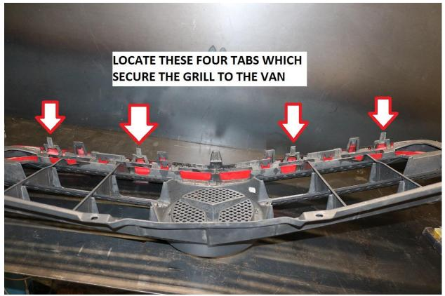
6) Once these tabs are located, push down on them and gently pull the bottom of the grill away from the van and it should easily come free from the vehicle. We have found a long flat nose screwdriver to work well as a tool to push down on the tabs.
