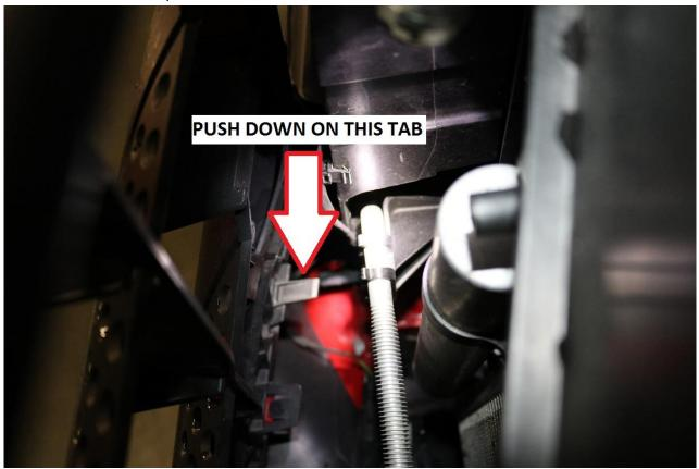
7) Locate the two push pin fasteners located near the front bottom side of the bumper cover which connects the inner fender well liner to the front bumper cover.
