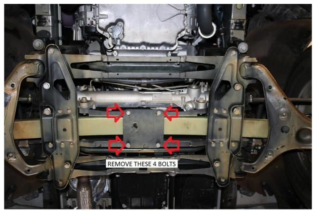
19) The main 401001-02 aluminum skid plate attaches to the vehicle via the factory holes noted in the image below. Take note of which holes will be utilized.
