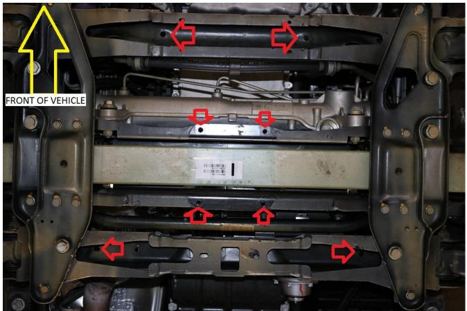
20) Raise the main aluminum skid plate into position. Try not to cover any of the mounting holes when raising it in place. Use a floor jack to lift into position.
