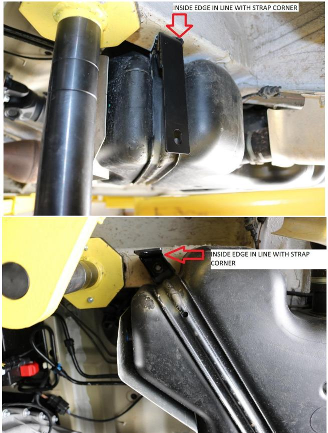
7) Make sure all bracket are parallel with the fuel tank sides, and torque all the OEM hardware to 40 ft-lbs (54 N.m).
