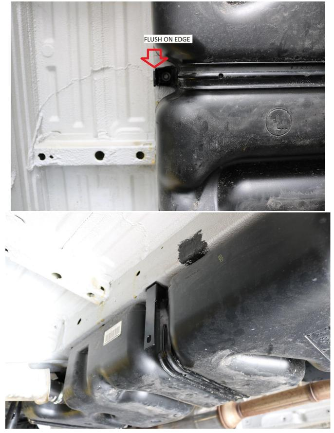
6) For the front angled brackets, line the inside edge up with the corner of the factory fuel tank straps.
