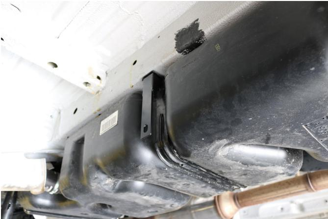
6) For the front angled brackets, line the inside edge up with the corner of the factory gas tank straps.
