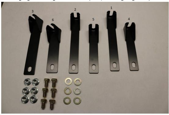
4) Install the brackets by loosening the mounting bolts in their corresponding locations. Loosen the bolts with an 11mm 12 point socket. Loosen the bolt enough to slide the brackets under the bolt head. Push up on the factory gas tank straps to fit the bracket between the straps and the bolt head.
