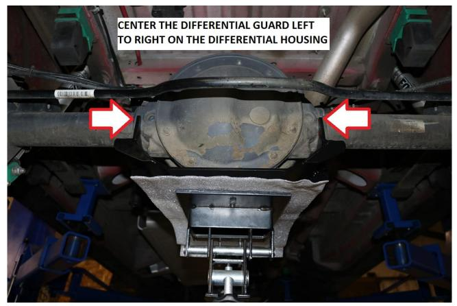
3) Take care when raising the differential guard into position that the front contact point does not contact or damage the pinion dust shield during installation.
