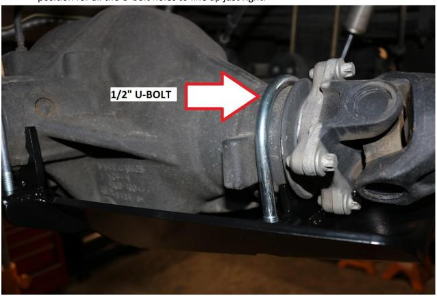
8) Install the included washers and nylock nuts on the front U-bolt. Snug the nuts on this U-bolt but again, do not fully tighten at this time. Use a ¾" socket for installation.
