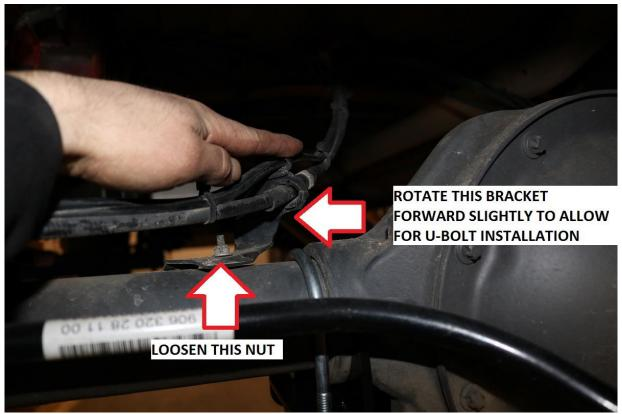
6) Once the 3/8" U-bolts are in place, install a washer and 3/8" nylock nut as pictured below. The nuts may be snugged down but do not fully tighten at this time. Use a 9/16" socket for installation.
