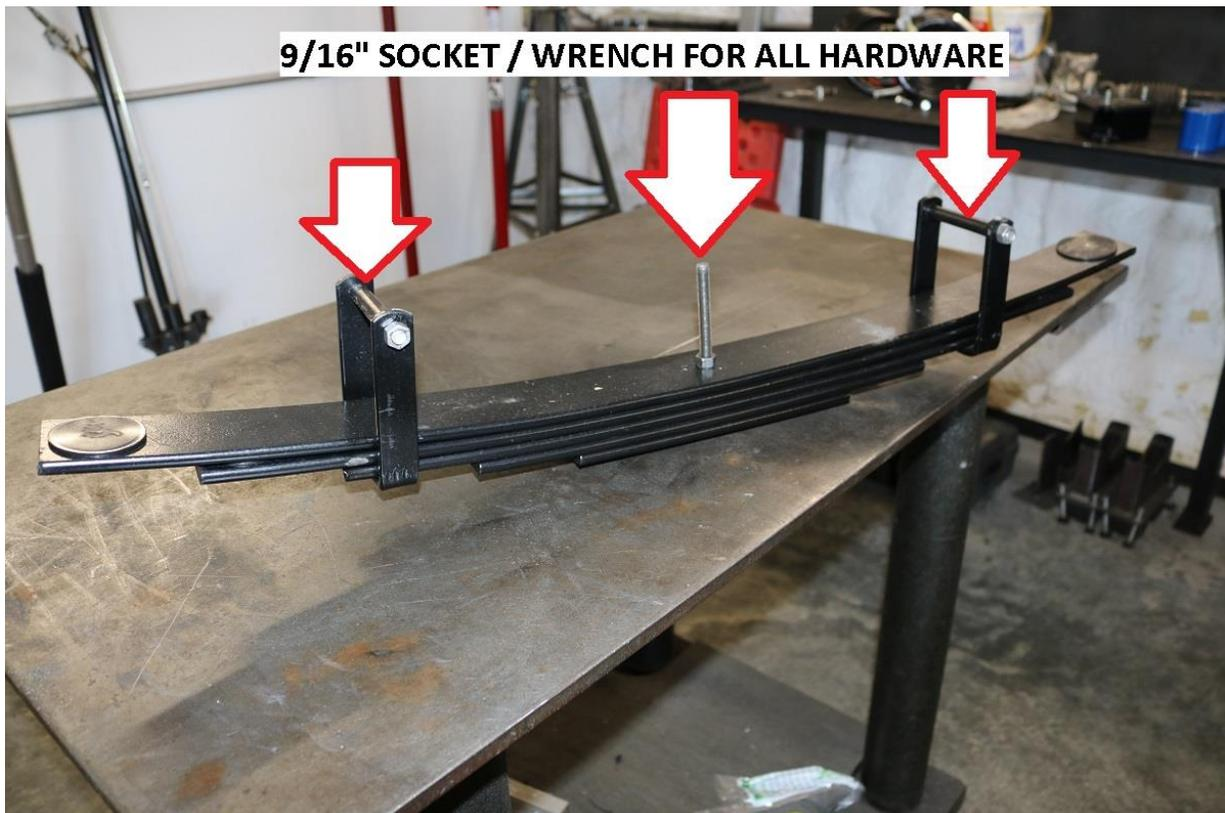
**14) CRITICAL:** A maximum of **3 leafs** can be installed per side without installing a full rear lift kit that includes bump stop drop brackets, extended sway bar links, and extended rear shock mounts.
