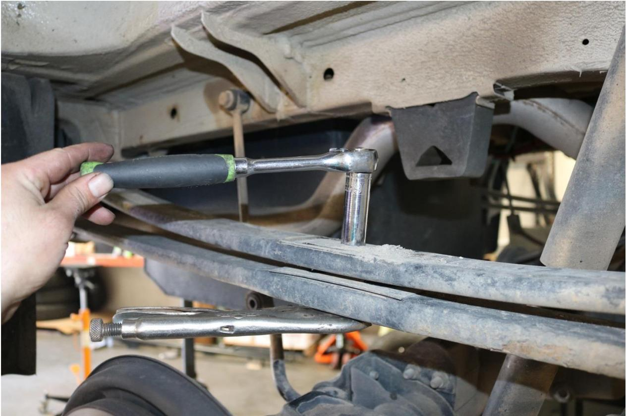
13) Next disassemble the mini pack by using a 9/16" socket / wrench to remove the leaf spring center pin nut and the bolt / nut for the spring clamps. Retain all hardware.
