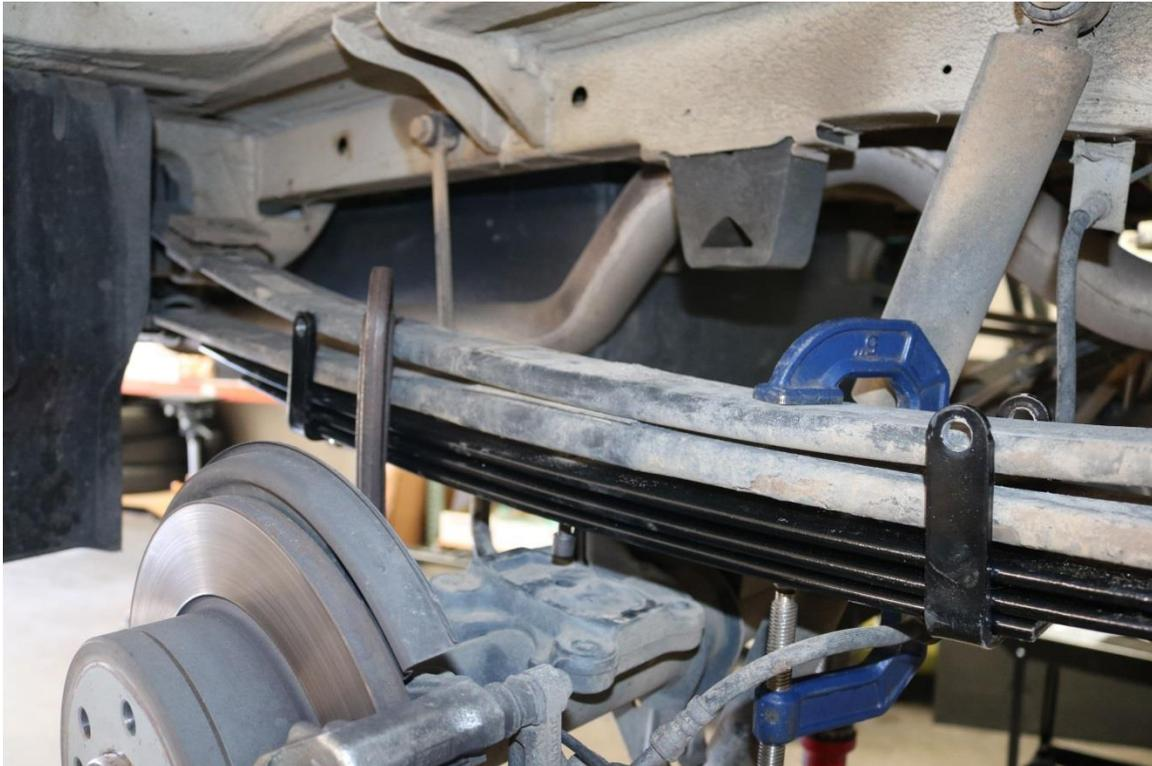
17) Once the springs are aligned and clamped all the way into position, install the 3/8" center pin nut removed in step 13 and tighten with a 9/16" socket / wrench. Torque to 22 ft-lbs (30 N.m)
